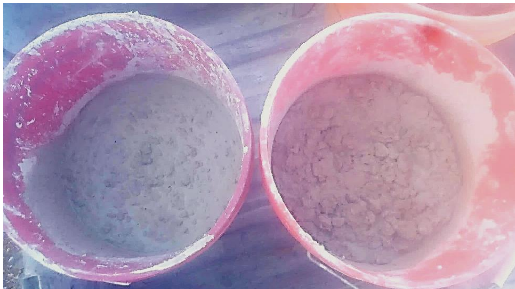
Figure 80: Consistency of Mixes with 11oz HRWR (left) and 9oz HRWR (right) after Final Slump Cone 3" Measurement and Being Vibrated.
