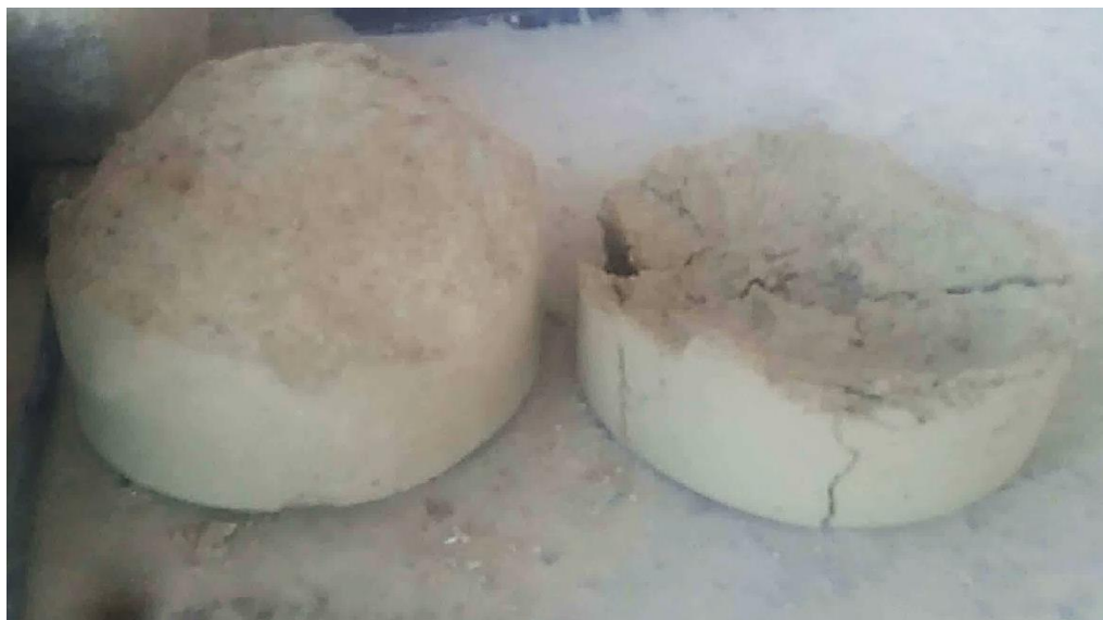
Figure 85: Splitting of Partially Set Bottom Portion of 0.30% Penetrometer Specimen
