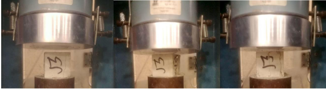
Figure 31: Series of Expansive BCSA Mortar Cubes Dosed with 0.2% Citric and Tested at 9 Days
