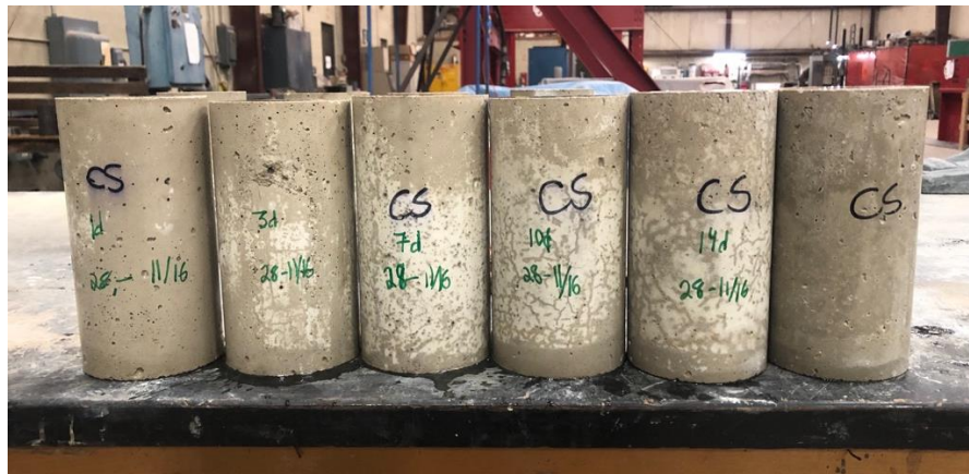
Figure 34: Shrinkage Cracking on Wet Cure Duration Compressive Specimens
