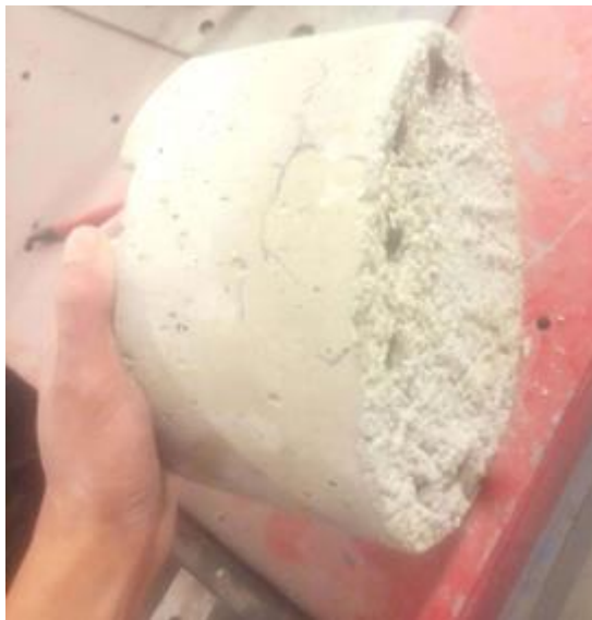
Figure 82: Angled View of Demolded Penetrometer Specimen Cracks
