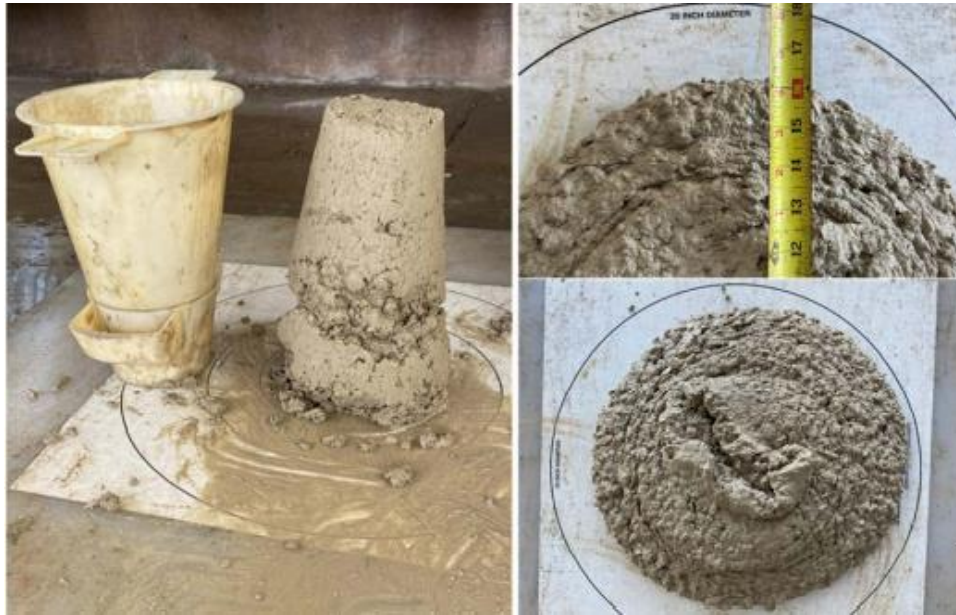
Figure 4: Slump Taken from Mix FR-1, Which Flash Set (left), and FR-2 (right), Where Citric Acid Retarder was Added to the Water Initially Soaking the Aggregate (Roswurm 2023)
