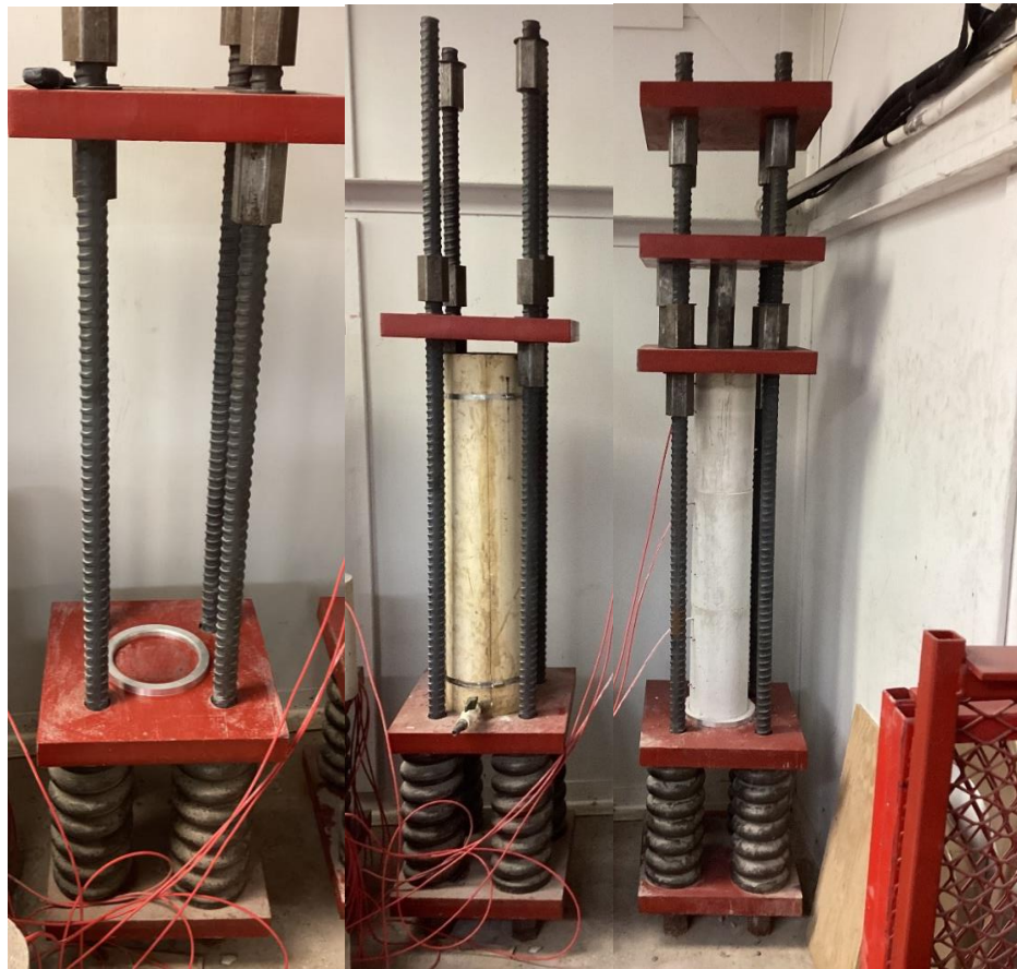
Figure 17a-c: (a) Unloaded Creep Frame with Spring Loaded Base and Centering Ring, (b) Creep Frame with PVC Standpipe in Place, (c) Loaded Creep Column after Draining and Removal of PVC Standpipe.
