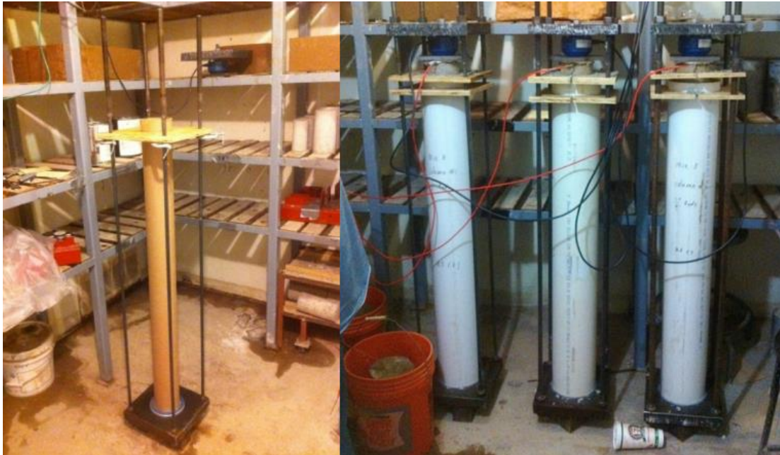
Figure 1: Cardboard Formwork and PVC Casing for Wet Curing (Roswurm 2013)
