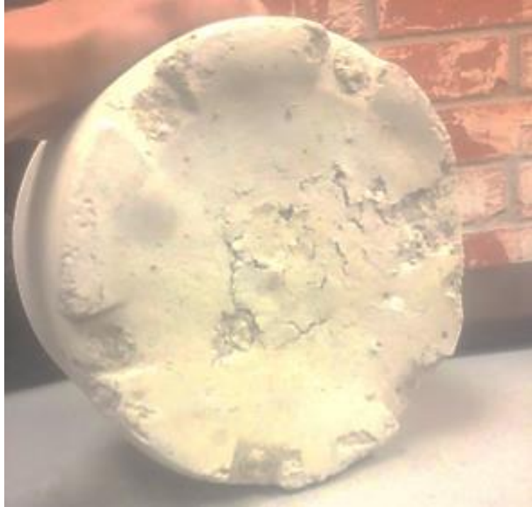
Figure 83: Damage to Bottom of Partially Set Demolded Penetrometer Specimens
