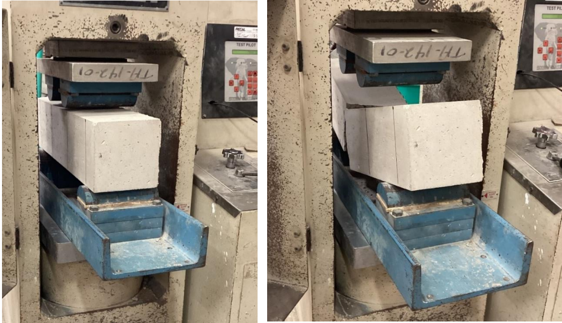
Figure 12: Modulus of Rupture Testing Set-up (left) and Failure Mode (right)
