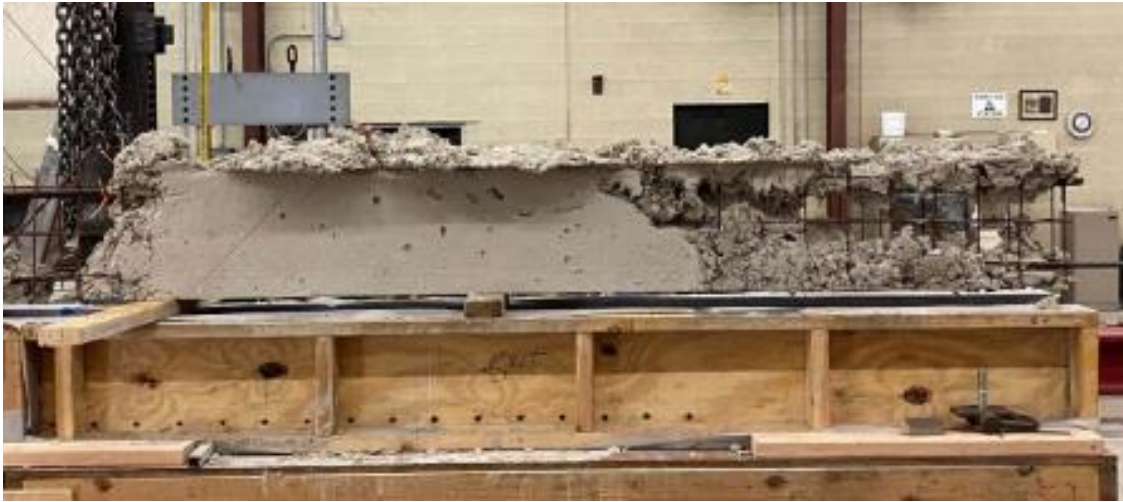
Figure 5: Side View of Flash Set Beam Specimen, B1.
