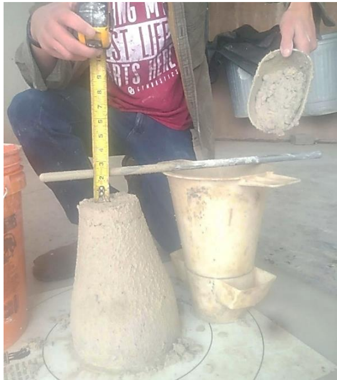
Figure 78: 2" Slump of Expansive BCSA Concrete at 2h after Cement Addition, vs Vibrated Scoop of Concrete.
