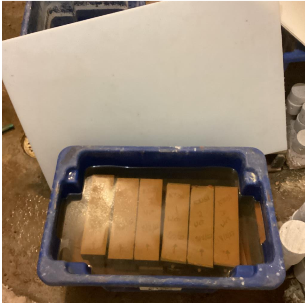
Figure 14: Plastic Tank Storing Wet Curing C157 and C878 Specimens, with Plexiglas Sheet Used to Cover Tank Behind
