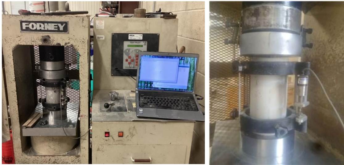
Figure 13: Set-up for Modulus of Elasticity Testing (left) and Testing Frame (right)
