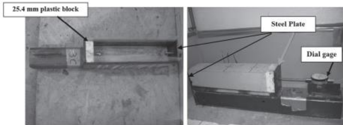
Figure 3: Mold and Testing Set up for Shrinkage from Zero Testing
