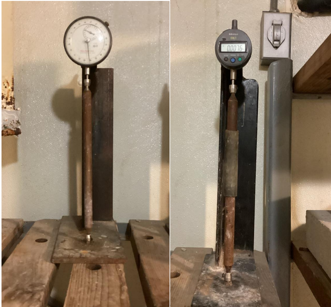
Figure 15: Comparators for Restrained (left) C878 and Unrestrained (right) C157 Shrinkage Testing
