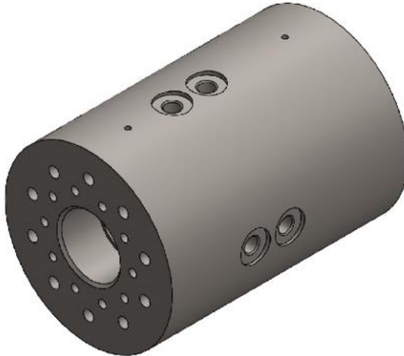
Figure 14: Horizontal Loading Pressure Chamber
