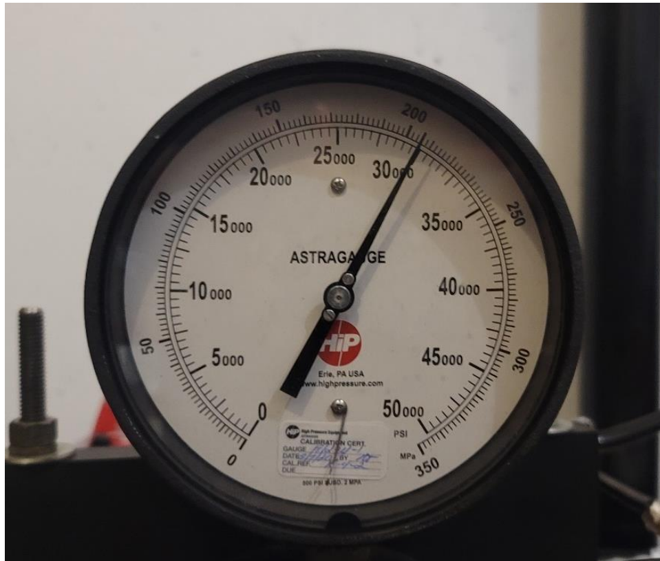
Figure 42: Proof Pressure Test Primary Pressure Gauge at Test Pressure - 30,000 psi
