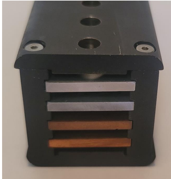
Figure 41: Coupon Holder Loaded with Material Coupons for Testing
