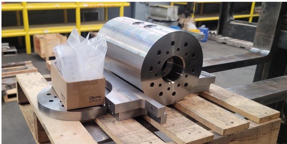
Figure 22: Uncoated Final Pressure Chamber Manufactured Components
