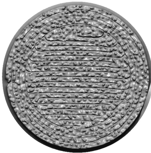
Figure 5. A TopMatch-GS scan of the bottom of the printed cartridge case that contacts the print bed. Multiple characteristics of the print bed that transferred to the bottom of the printed object can be easily observed.
