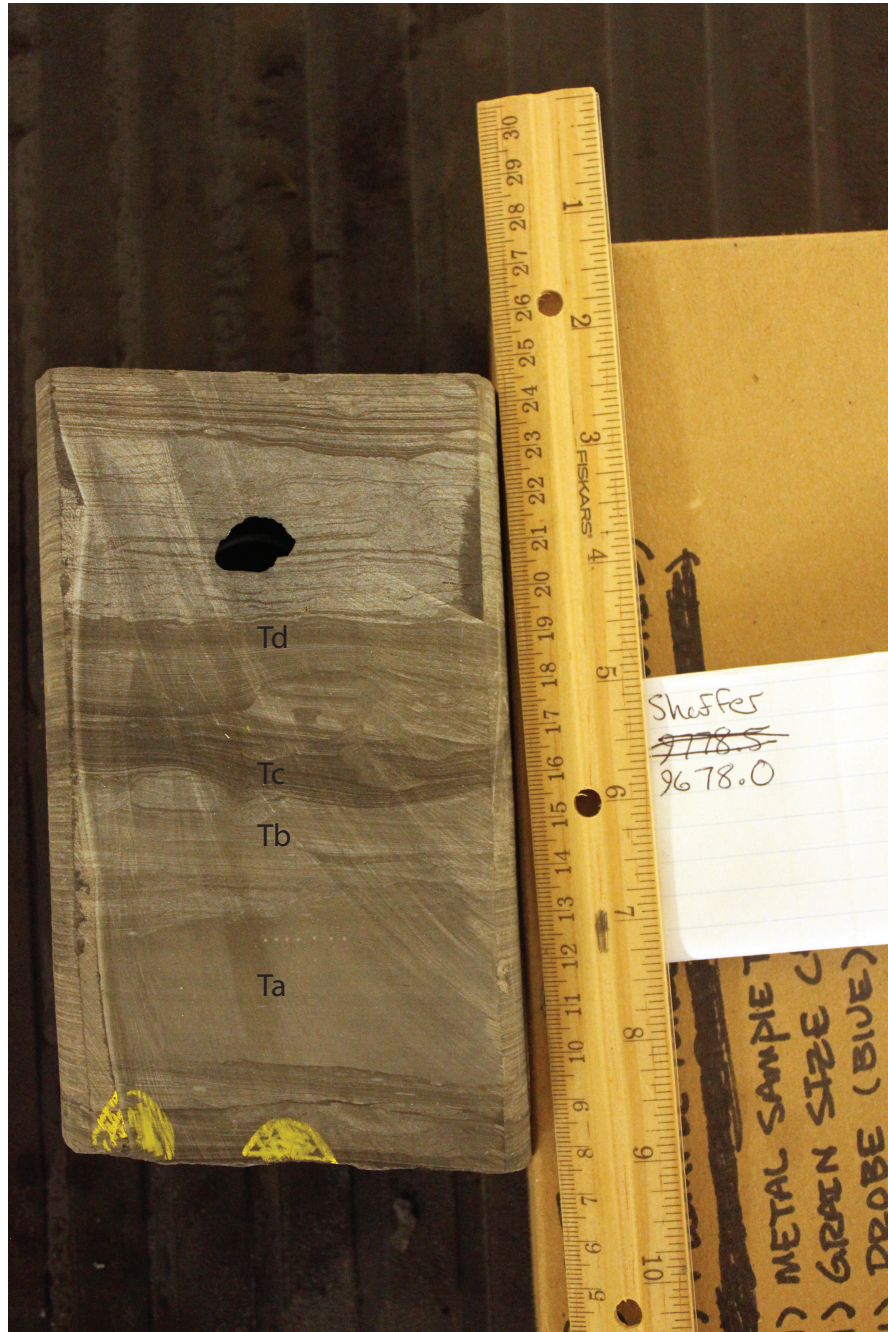
Figure E-6. Possible Bouma sequence in Shaffer 1-23 consisting of, from base to top, structureless calcareous siltstones (Ta), parallel-laminated siltstones (Tb), wavy laminated argillaceous siltstones (Tc), and faintly-laminated mudstones (Td). These fining-upwards sequences increase in clay content and decrease in carbonate content from base to top.
