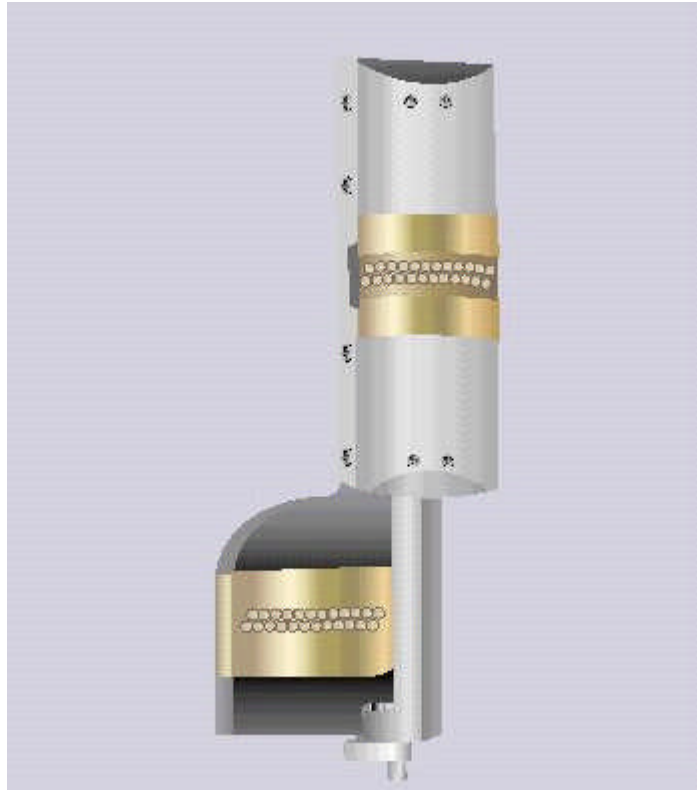
Figure 1.1. Pad and flap assembly of the Formation MicroImager™ tool showing horizontally offset rows of electrode buttons (Schlumberger, 2002).
