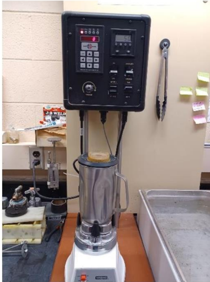
Figure 7: Laboratory mixer used for mixing cement slurry
