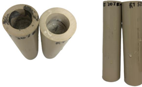
Figure 8: Customized pipes used for curing the cement samples
