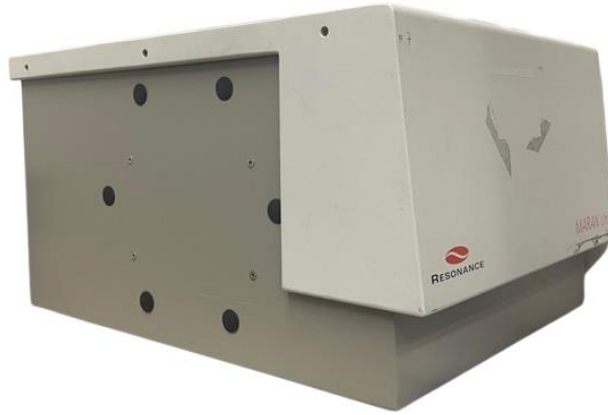
Figure 12: Bench-top Nuclear Magnetic Resonance (NMR) device used for measuring porosity
