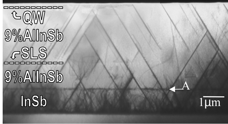
Figure 2.11: 220 DF X-TEM image taken from a [\bar{1}10] cross sectional specimen. Label A indicates the first InSb/Al 0.09 In 0.91 Sb interface from the GaAs substrate.
