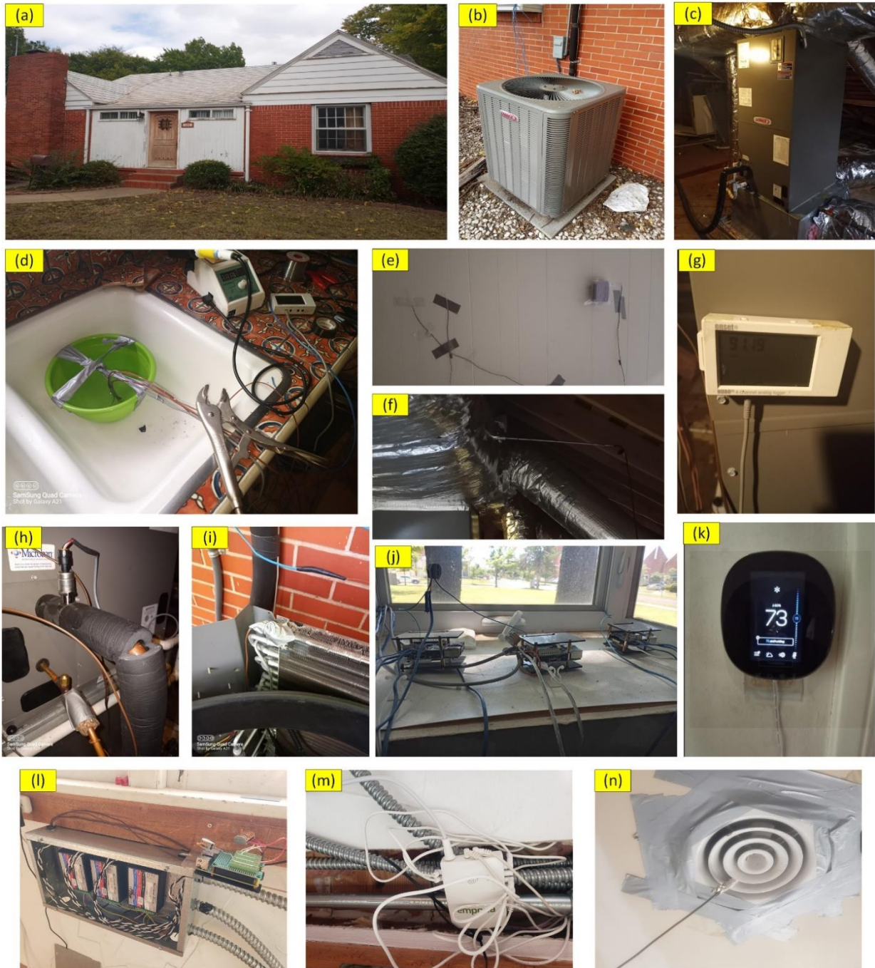
Figure 2.2: OU Lab-house overview (a) front view (b) Outdoor unit (c) Indoor unit (d) Thermocouple calibration (e) Tie Thermocouples (f) Indoor air velocity sensor (g) Hobo logger for SAT (h) condenser outlet temperature thermocouple (i) condenser saturation temperature thermocouple (j) Raspberry pi with mounted hat (k) Smart thermostat (l) Power meters (m) Smart power meter (n) Diffuser with a node sensor above it
