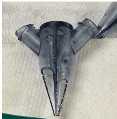
Figure 22: Tri-view of a Single-Printed Nozzle Removed from Build Plate
