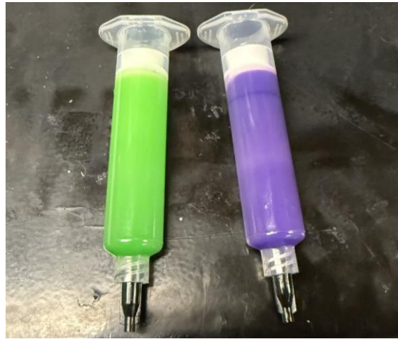
Figure 6: Side-by-side curing of the two silicone formulations used in dual-material printing: EcoFlex 00-30 and THI-VEX additive with green food coloring (left) and with purple food coloring (right)
