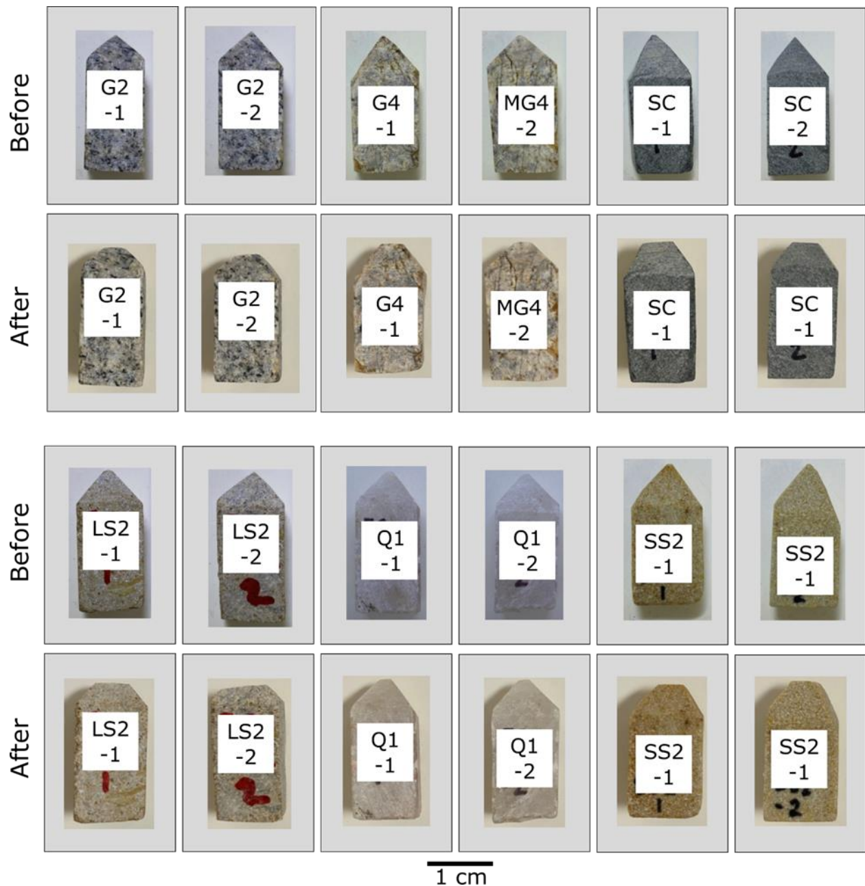
Figure 2. A selection of representative styluses before and after experimental glacial abrasion. Styluses are approximately 1 cm wide and 3 cm tall. The full catalog of before and after images for all styluses is in Appendix 1.
