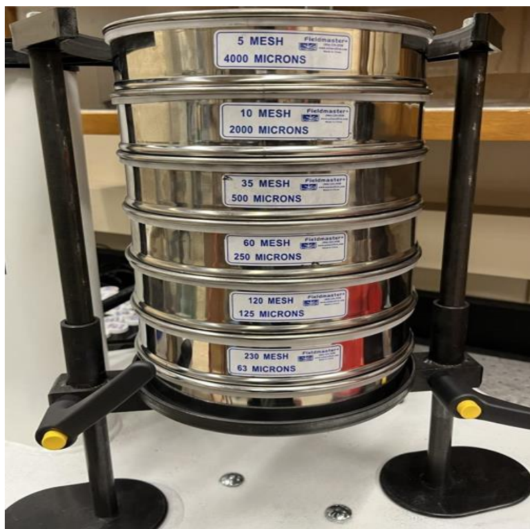
Figure 3.3: The arrangement of multiple sieves stacked within a sieve shaker with decreasing sieve openings from top to bottom.
