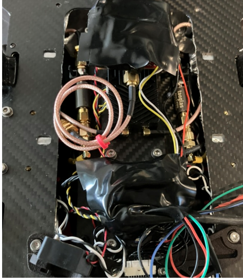
Figure 4.3: Example of “Level II” HIRF/EMI mitigation, focusing on protecting the C2 link and RF channel.
