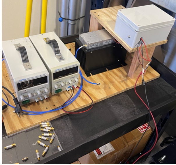
Figure 5.2: Example images of the laboratory test setup - Noise generation as RFI source.
