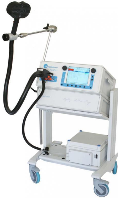
Figure 2-1: rTMS device from MagVenture, with a stand to hold the stimulator and a coil to deliver the stimulation (picture copyright by https://www.magventure.com/us ).
