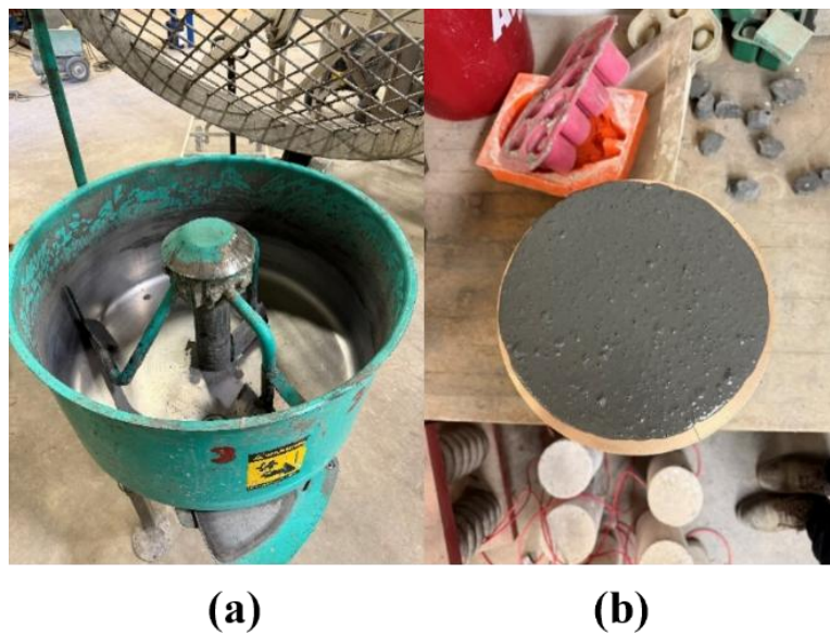
Figure 2.1: (a) Pan mixer (b) Flow test of UHPC with LWS
