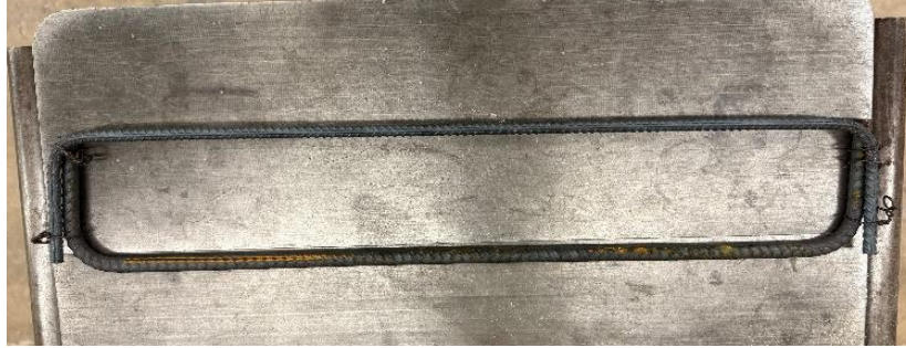
Figure 3.8: Top and bottom reinforcement prepared for placement in the beam specimens
