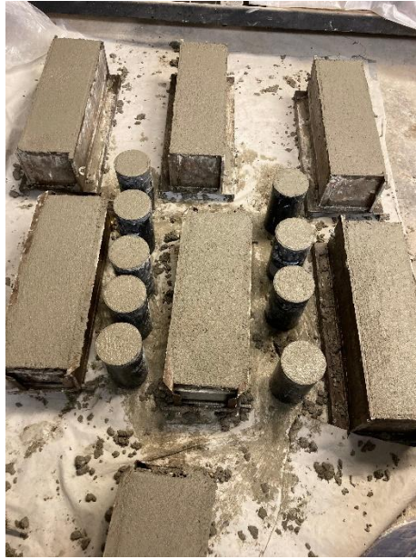
Figure 5.1: 6 in. x 6 in. x 21 in. specimens along with 4 in. x 8 in. cylinders
