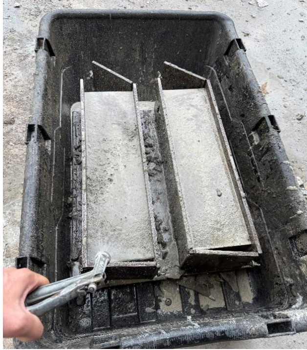
Figure 3.12: Washing the surface of concrete to expose aggregate following the setting time
