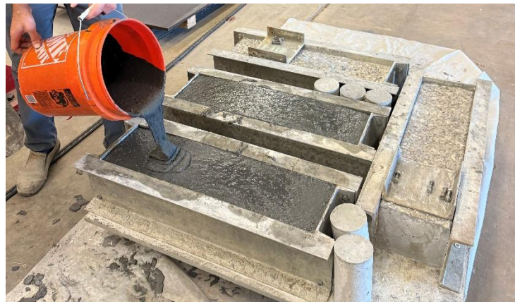
Figure 3.16: Casting UHPC overlay for 8 in. x 8 in. specimens
