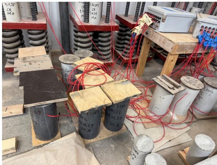
Figure 4.24: Shrinkage Measurement Using VWSGs
