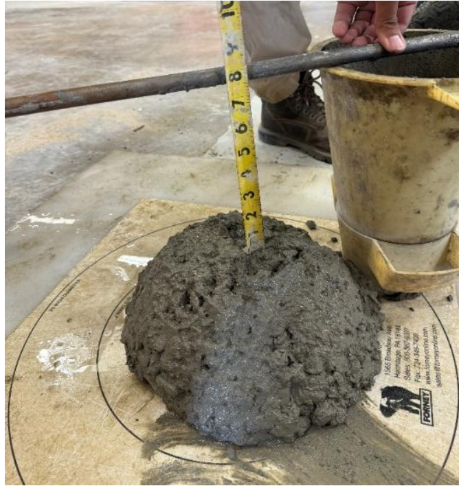
Figure 3.10: Representative slump test for the Class AA bridge deck concrete
