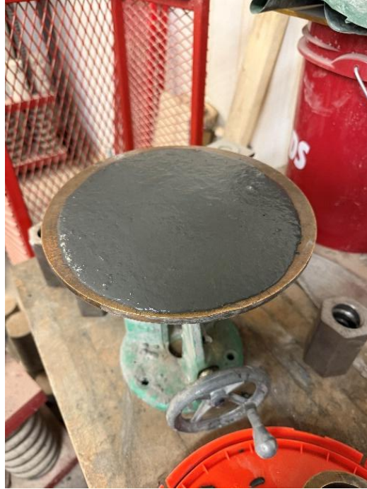
Figure 3.14: First UHPC overlay flow test
