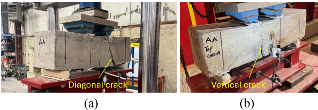
Figure 3.22: Failure of 8 in. x 8 in. x 30 in. No Overlay beam specimens with (a) No. 4 bar at the bottom and No. 3 bar at the top (positive moment) and (b) No. 3 bar at the bottom and No. 4 bar at the top (negative moment)
