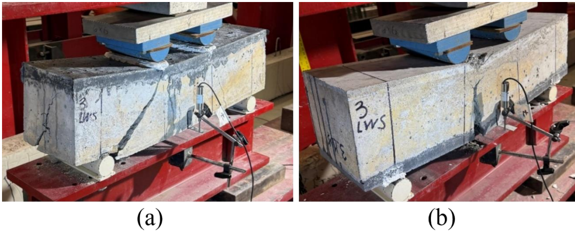
Figure 3.27: Failure of 8 in. x 8 in. x 30 in. UHPC-3 LWS overlay beams with (a) overlay in compression and (b) overlay in tension
