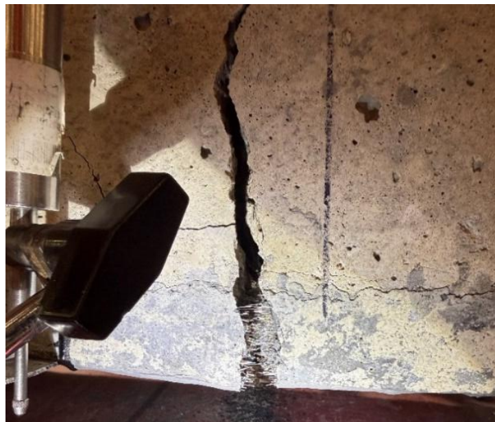
Figure 3.24: Fibers bridging the crack in the UHPC in an overlay tested in tension
