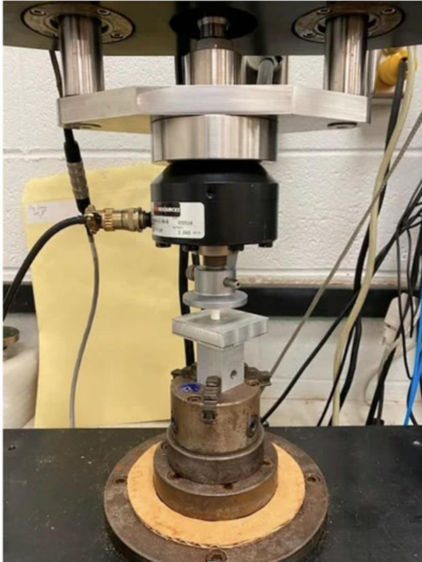
Figure 23. Compression test of a round PCL sample (diameter 9.8 mm and 7.8 mm height) in a Test Resource Universal Testing Machine
