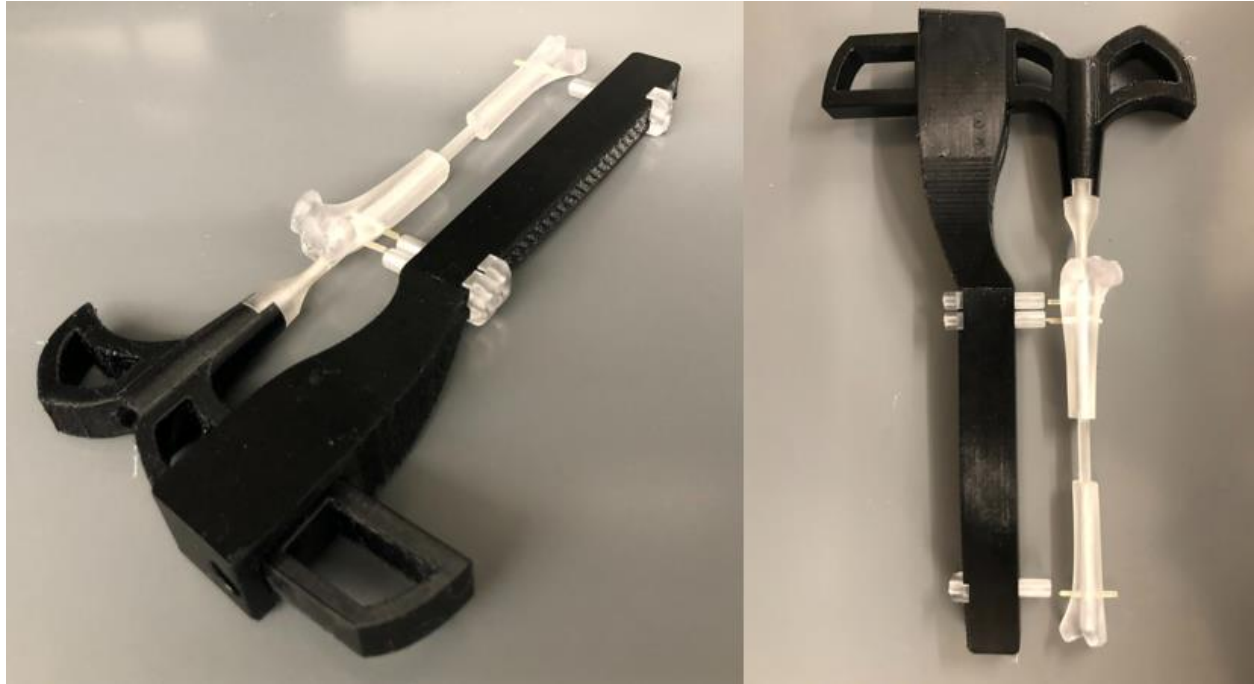
Figure 28. (a) The 3D printed targeting jig. (b) Efficacy tests of the fabricated delivery jigs using a 3D-printed rabbit tibia model, demonstrating the jig's capability to install an intramedullary nail and screws into a 20 mm-long rabbit tibia defect
