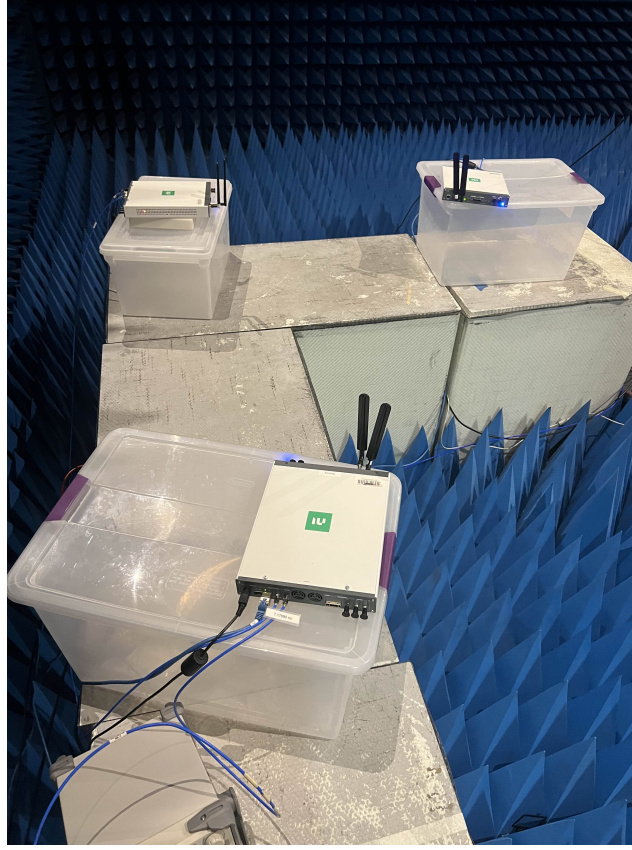
Figure 4.15: Over-the-air synchronization setup in an anechoic chamber for evaluating synchronization parameter estimation.
