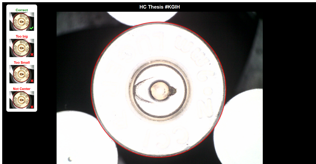
Figure 7: image of edge. Brightness intensity is automatically selected from BIQ and is increased to better visualize edge.
