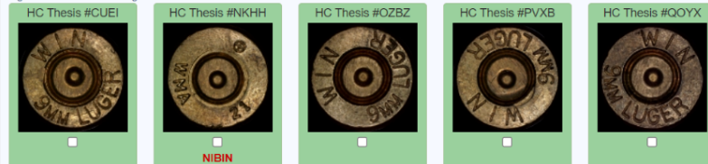
Figure 14: image of the results from the rotation effects during the experimental design. Utilized are five (5) cartridge cases with Winchester ammunition.
