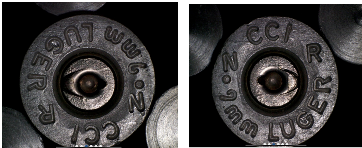
Figure 9: image of the drag mark changed from 3 o'clock to 9 o'clock & the ejector mark changed from 11 o'clock to 4 o'clock.
