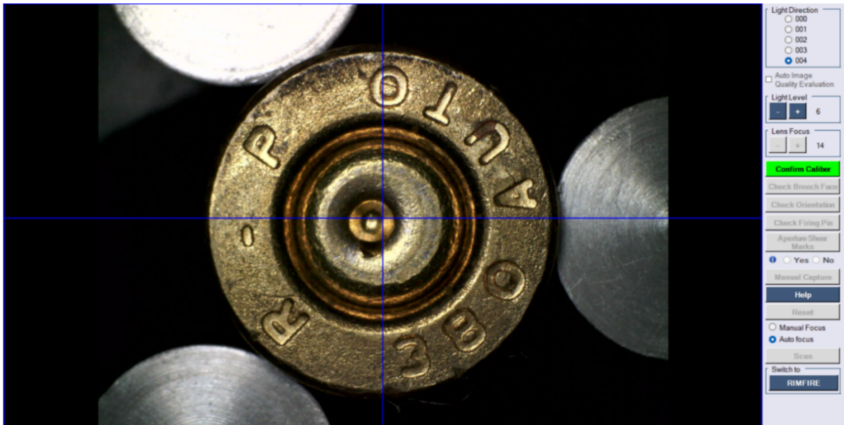
Figure 4: image of process prior to scanning cartridge cases. Involves confirming Caliber, Breech Face, Orientation, Firing Pin, & Aperture Shear Marks
