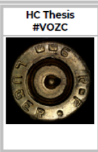
Figure 31: image of five (5) cartridge cases from Remington ammunition that were shot using the SCCY CPX within this study. Four (4) cartridge cases, GDYL, TTZN, ZYOQ, and SGDN, originated from the same firearm. Three (3) cartridge cases, GDYL, TTZN, and ZYOQ, at a high confidence and one (1), SGDN, at a low confidence. One (1) cartridge case, VOZC, was labeled as undetermined.
