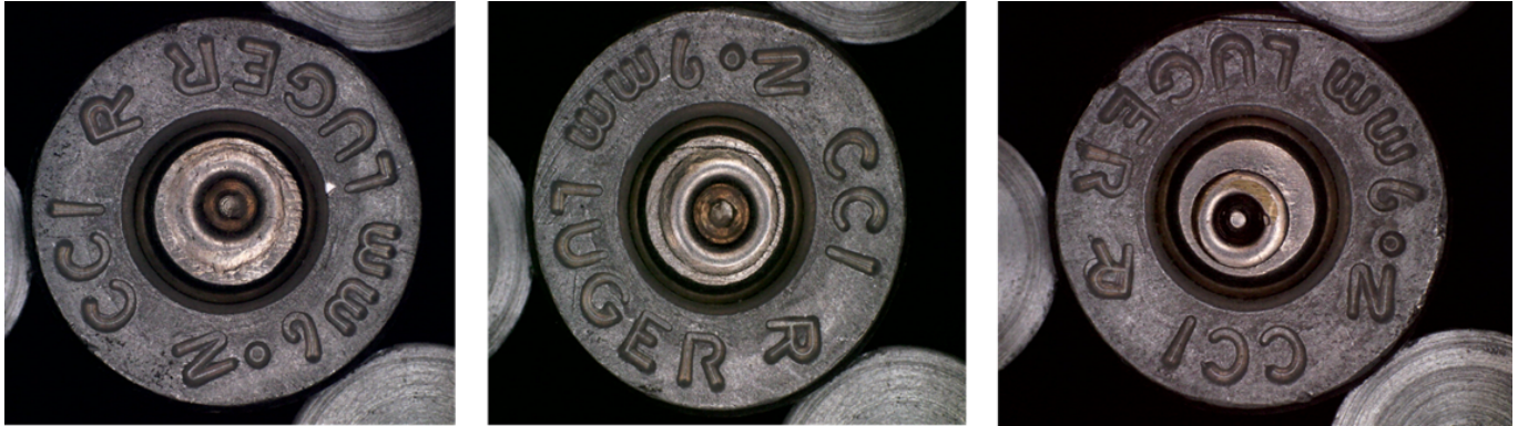
Figure 25: Image of three (3) cartridge cases, one from each firearm involved in the CSA Triage report for Firearm #5. The left cartridge case is labeled as HYEQ in the BIQ database and originated from a Taurus PT92. The middle cartridge case is labeled as NLAW in the BIQ database and originated from a Beretta 92FS. The right cartridge case is labeled as SOKE in the BIQ database and originated from a Ruger P89.
