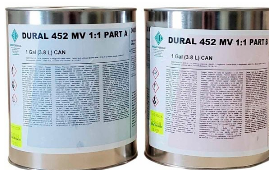
Figure 2. Dural 452 MV 1:1 resin and hardener.
