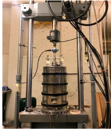
Figure 8. Setup for resilient modulus test.
