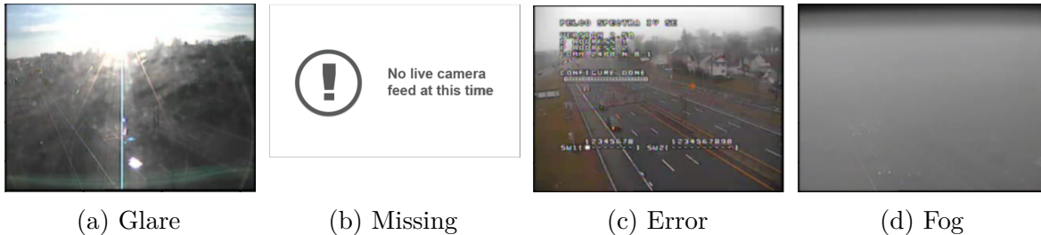
Figure 5.8: Four examples of conditions that are present in the unlabeled data that correspond to input types that are not represented in the labeled training data. Some conditions only present in the unlabeled data can obscure the road surface making it impossible to determine its condition.
