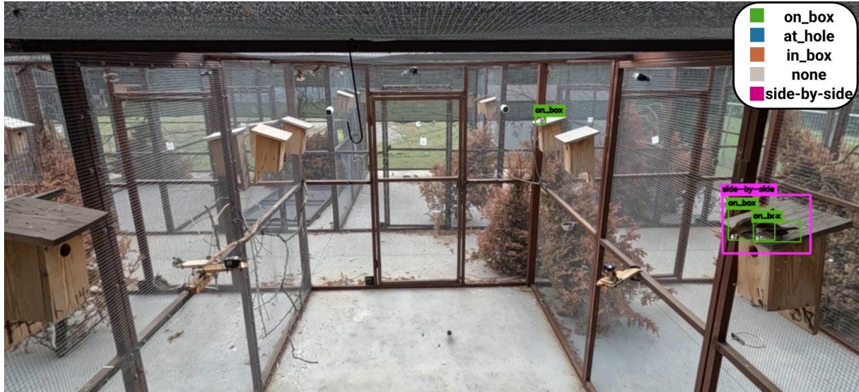
Figure 5.7: Sample annotated frames from the visualization layer with side-by-side interaction detection. A combined interaction bounding box (magenta) is drawn around the interacting pair once the bout is confirmed over a minimum of 90 consecutive frames at 30 fps.
