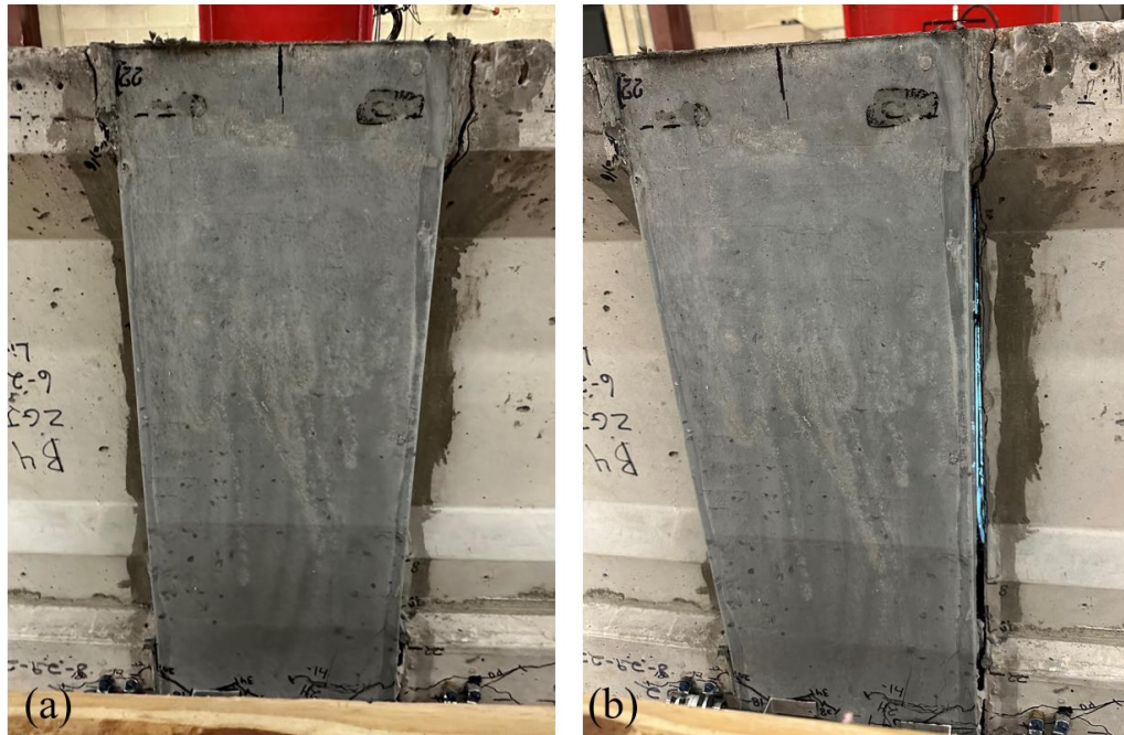
Figure 64: West (a) and southwest (b) side of HSDU-2 showing separation at the interface after negative moment testing
