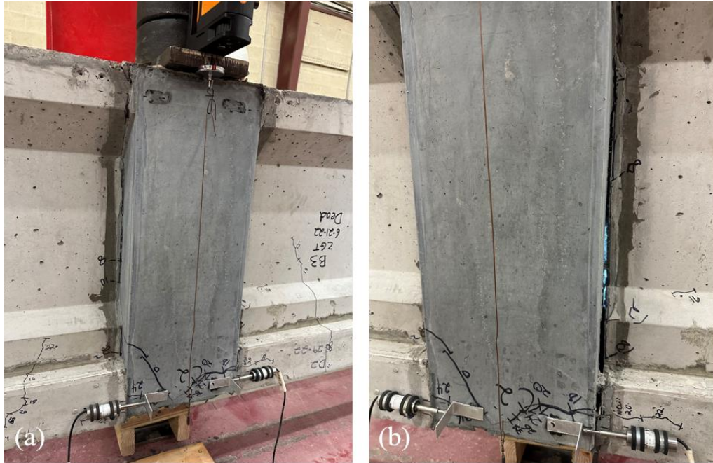
Figure 52: Northwest (a) and southwest (b) side of joint HSDU-1 under final negative moment test loading
