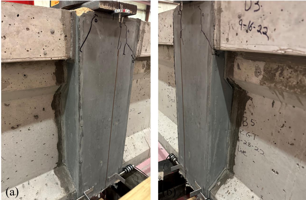
Figure 72: Southeast (a) and northeast (b) side of joint SSDU-1 showing the joint interface before positive moment testing
