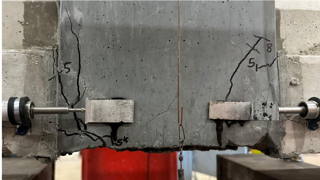
Figure 96: West side of joint SSDU-2 showing cracks near the as-cast top face of the joint under final negative moment test loading
