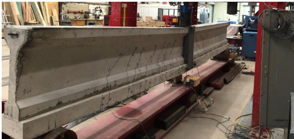
Figure 28: HSJ3-1 entire specimen showing deflection under final loading
