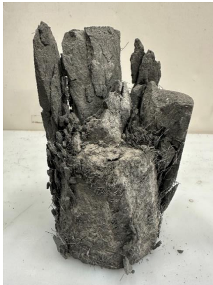
Figure 68: Compressive cylinder showing significant fiber settlement in the Ductal® UHPC used for joints HSDU-1 and HSDU-2
