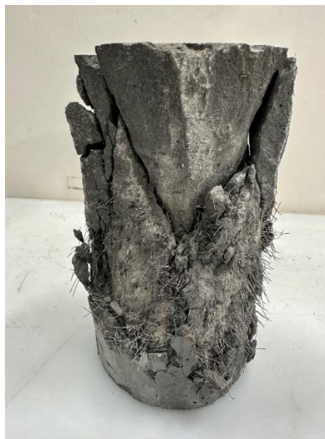
Figure 79: Compressive cylinder showing significant fiber settlement in the Ductal® UHPC used for joints SSDU-1 and SSDU-2
