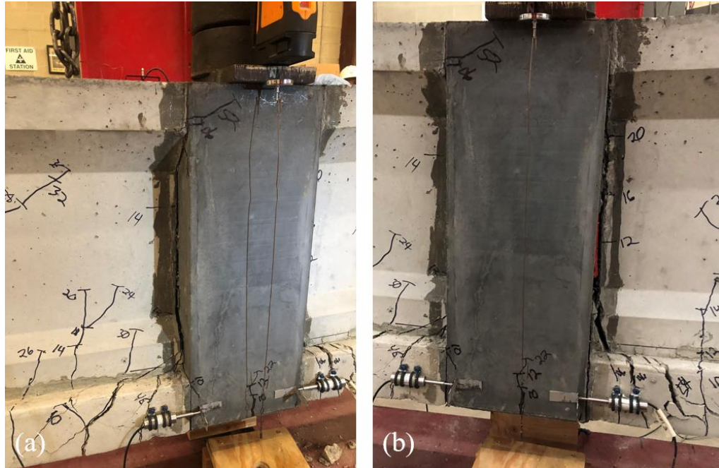
Figure 27: Northwest (a) and southwest (b) side of the joint HSJ3-1 under final loading
