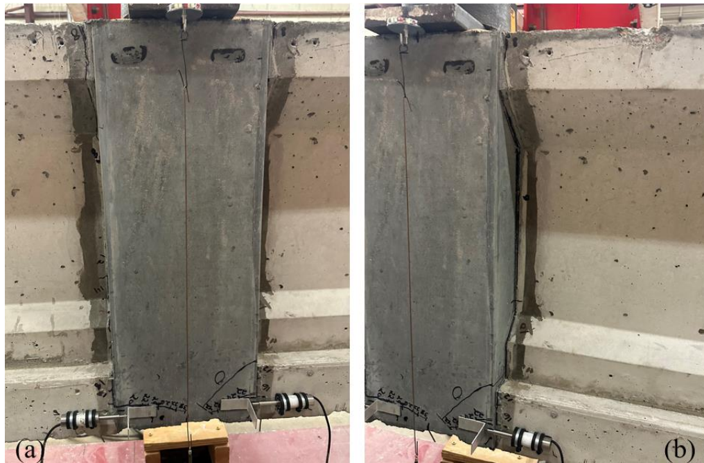
Figure 50: East side of the joint (a) and northeast side of the interface (b) of HSDU-1 before negative moment test
