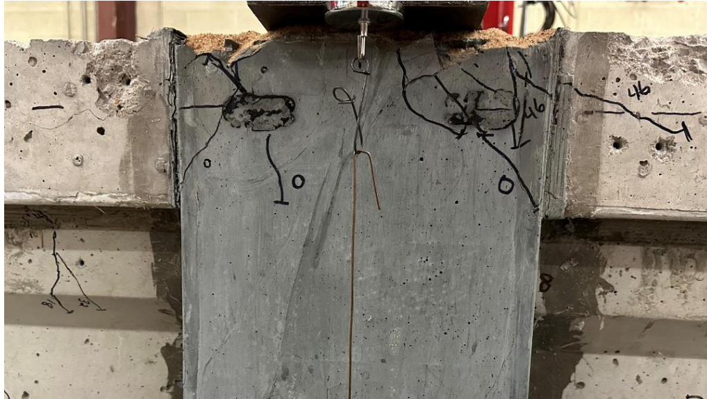
Figure 101: East side of joint SSDU-2 in positive moment orientation showing undocumented cracks near the as-cast top surface caused by negative moment testing Note: All cracks unlabeled or labeled 46 kips resulted from final loading of approximately 41.6 kips
