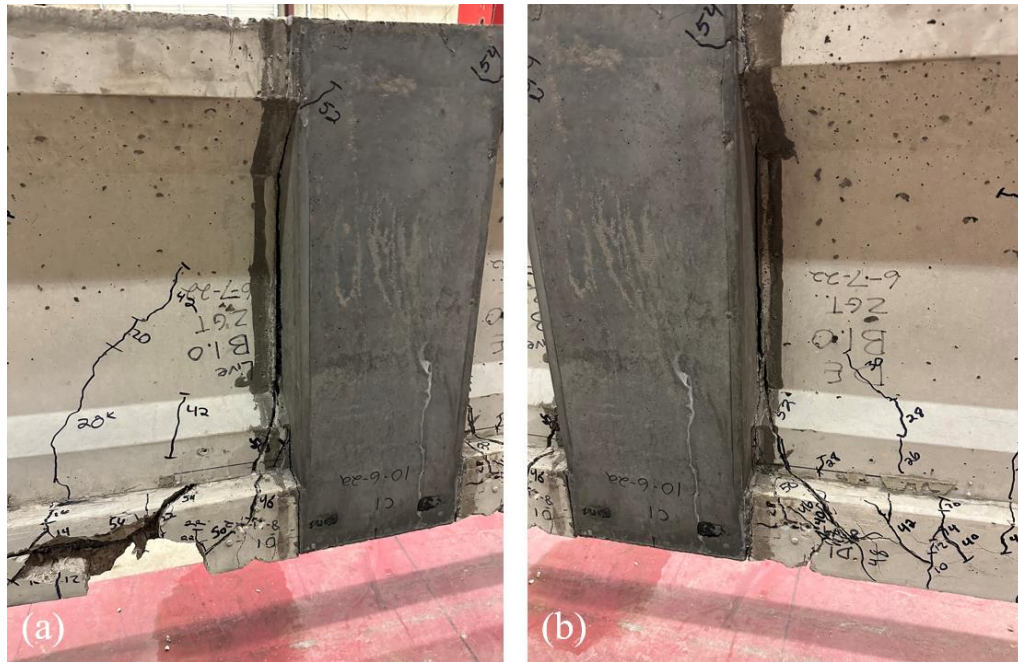
Figure 29: Southeast (a) and northeast (b) side of joint HSJ3-1 after final loading
