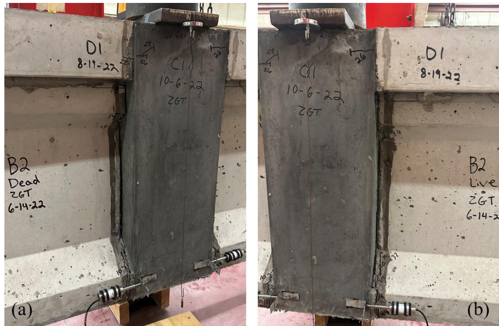
Figure 34: Southeast (a) and northeast (b) side of the joint HSJ3-2 after testing
