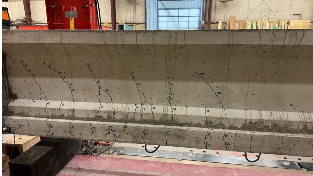
Figure 82: East side of north girder SSDU-1 showing flexural cracks after negative moment test
