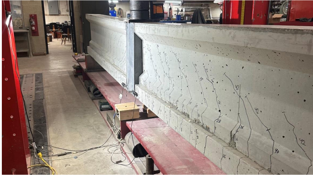
Figure 41: Visible deflection and additional flexural cracking of HSJ3-2 under final loading
