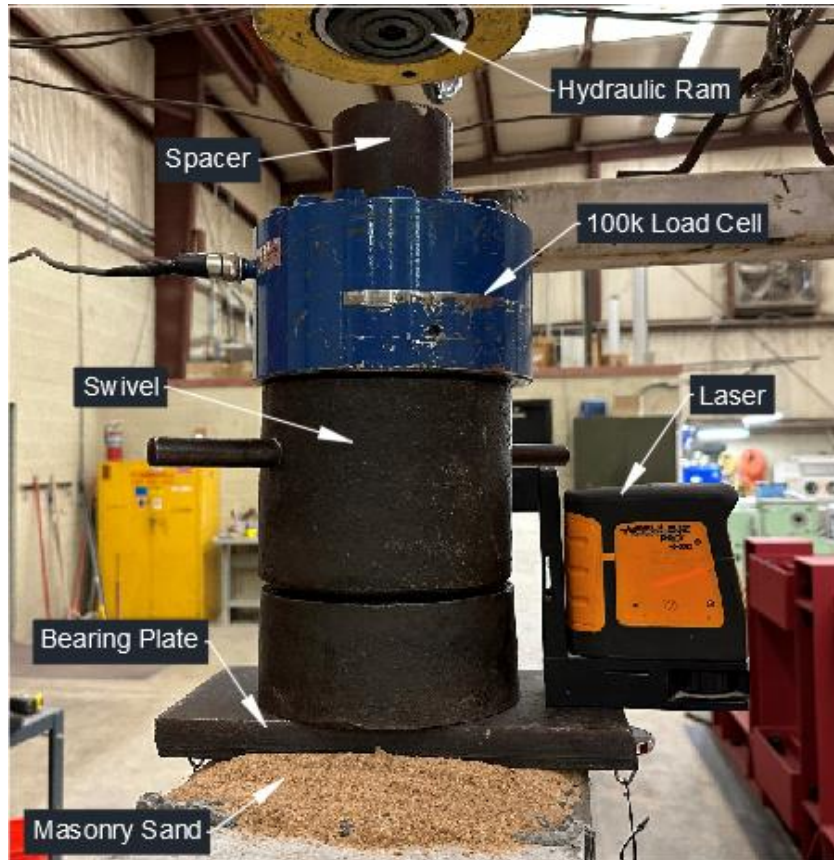
Figure 25: Detailed view of components for joint testing apparatus
