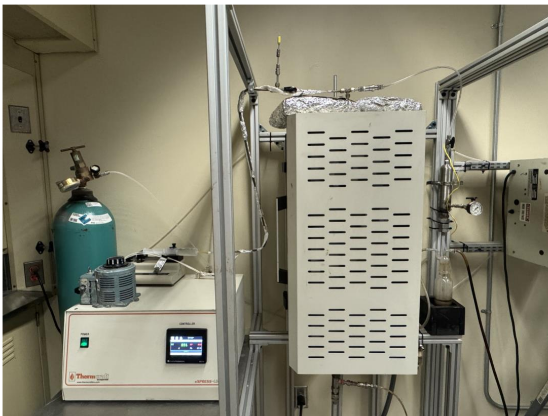
Figure 10: Experimental setup for investigating biomass conversion processes: pyrolysis and gasification.
