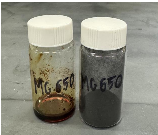
Figure 13: Bio-oil (left) and biochar (right) collected during the biomass conversion process.
