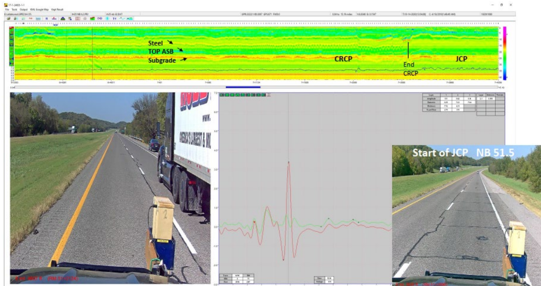
Figure 2.7 GPR Analysis on I-35 Northbound Mile 51.5
