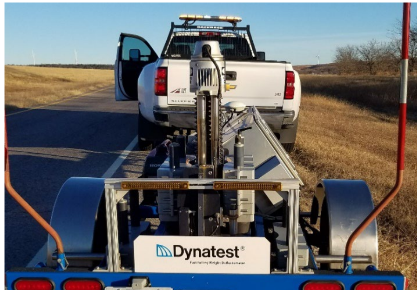
Figure 4.1 Falling Weight Deflectometer Measurement Approach (116)
