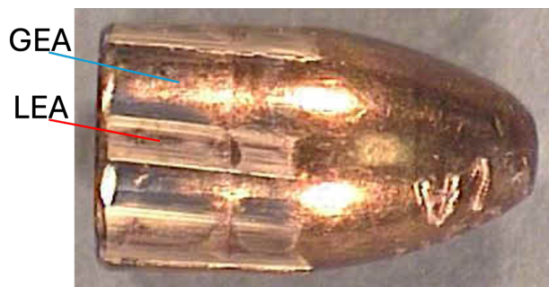
Figure 1.2: Fired bullet depicting both LEAs (shown in red) and GEAs (shown in blue).
