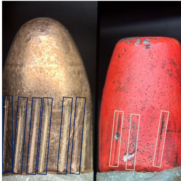
Figure 1.10: comparison of a fired FMJ projectile showing identifiable striations (highlighted in blue boxes), and a fired TSJ projectile, which exhibits uniform pitting and partial surface melting (highlighted in gray boxes)
