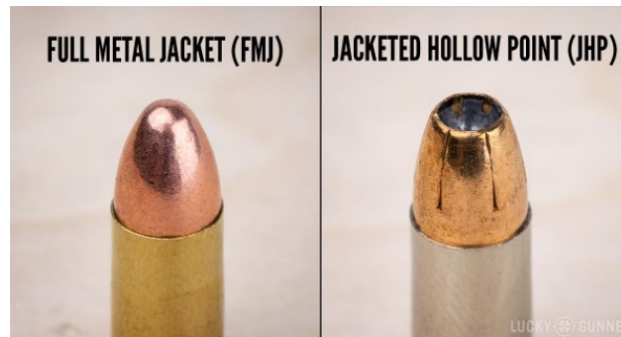
Figure 1.8: Comparison between Full metal jacket (FMJ) and Jacketed hollow point (JHP) ammunition.
