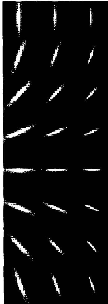
Fig. 2.6: A Gabor filter set with three different scales and eight different orientations is shown. The scales are set by changing the standard deviation of the Gaussian function, while the orientations are obtained by changing the angle of the sinusoid.
