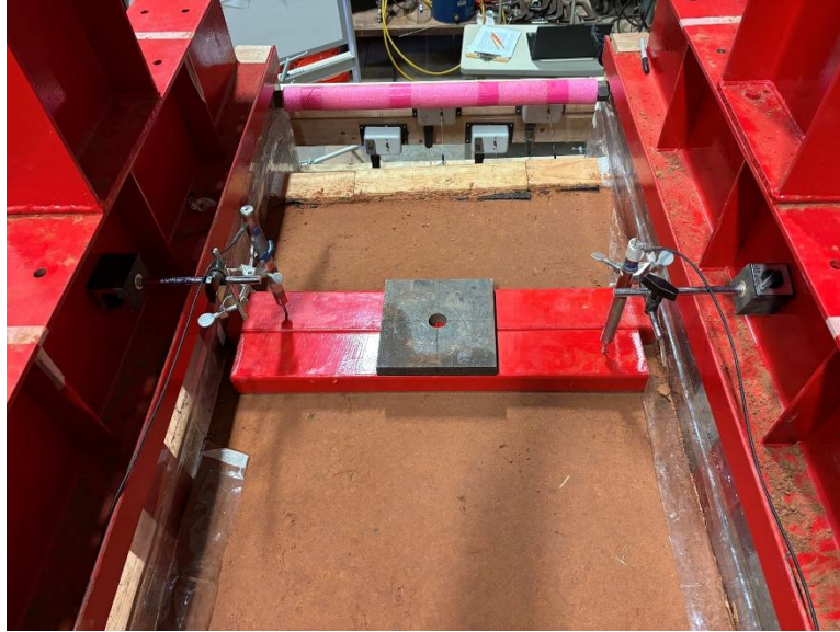
Figure 5.2 LVDTs were used to measure strip footing settlement
