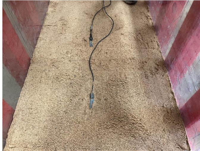
Figure 5.1 Placement of EC5 sensors before the next lift
