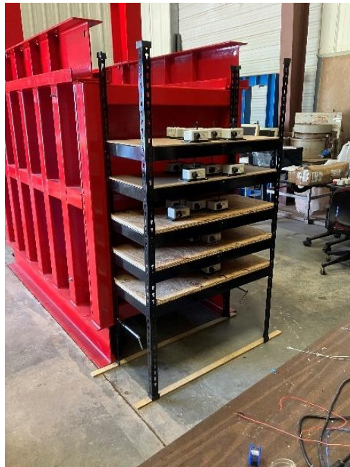
Figure 5.9 Wire potentiometers (WPs) at the back of the test box
