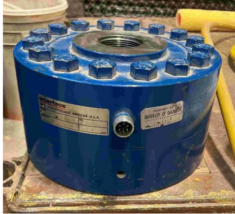
Figure 5.5 Load cell used in the model tests
