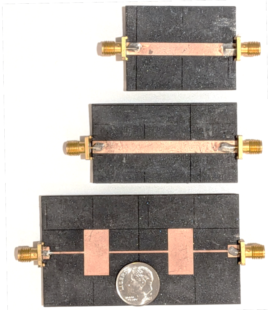
Figure 6.9: Fabricated two-port microstrip structures on MX substrate. (Top) 45 mm TL (Middle) 60 mm TL (Bottom) 81.7 mm TL (d) 5th order LPF
