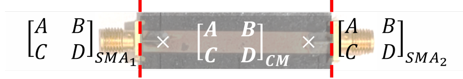
Figure 6.12: Cascaded ABCD -matrices overlaid on a microstrip TL. The region for each matrix is divided by a red dashed line.
