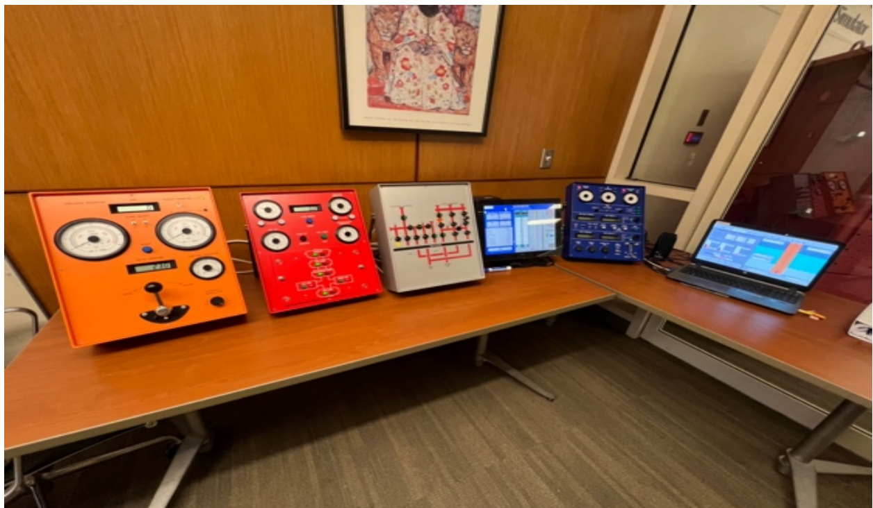
Figure 4.2.2 The DrillsIM50 Portable Well Control Simulator (OU Simulation Lab)
