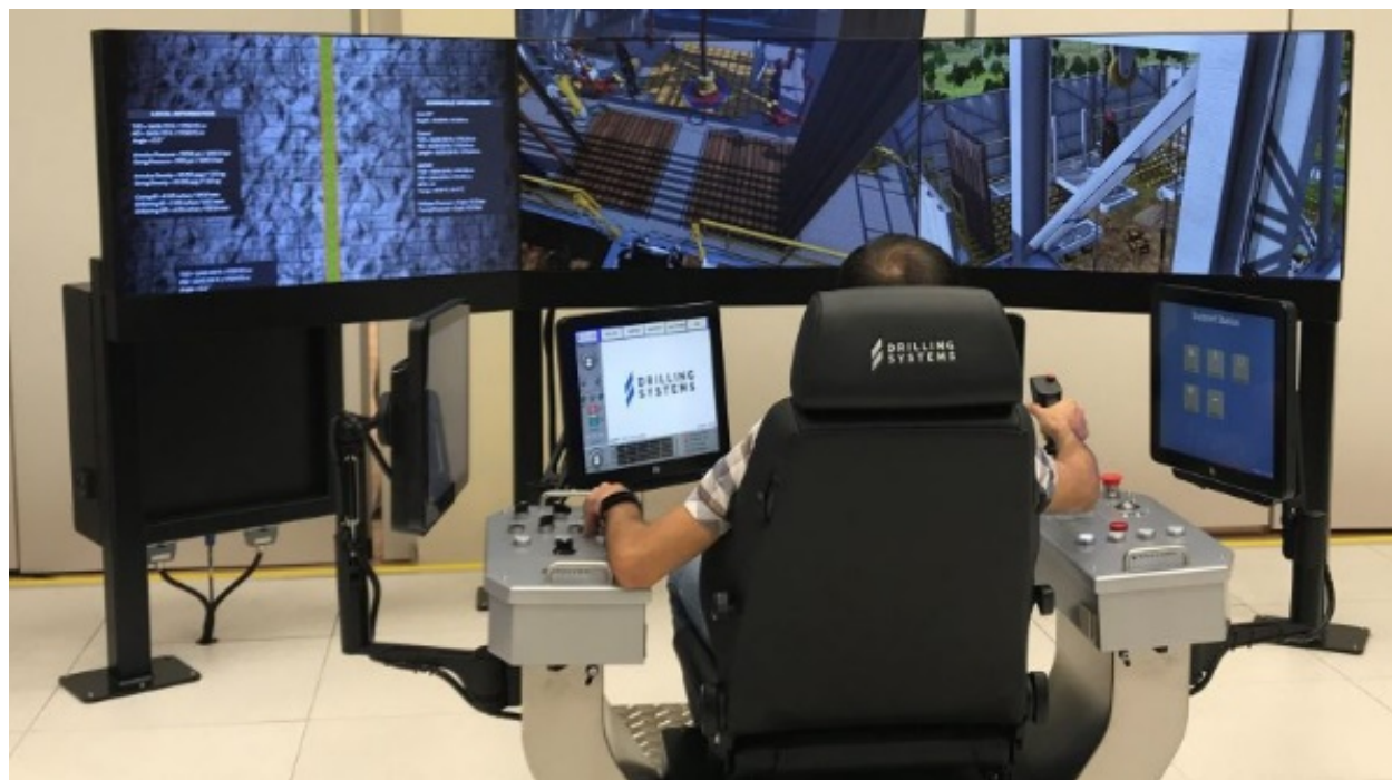
Figure 4.3.2 The full-size cyber drilling and well control simulator (Drilling systems 2022)
