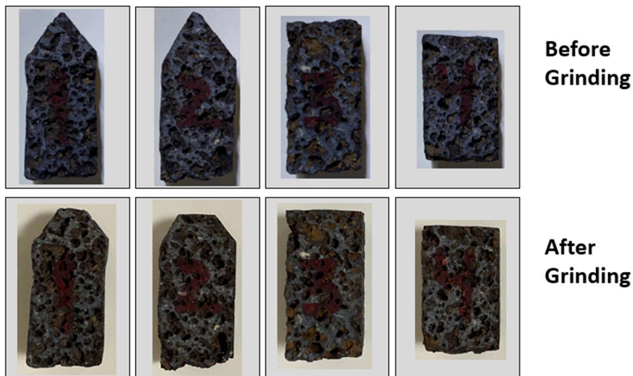
Figure A5. Sample series MG5 clasts before and after grinding. Clasts on the top row are before grinding, and clasts on the bottom row are after grinding. Clasts are approximately 1 cm wide and between 2 and 3 cm tall.
