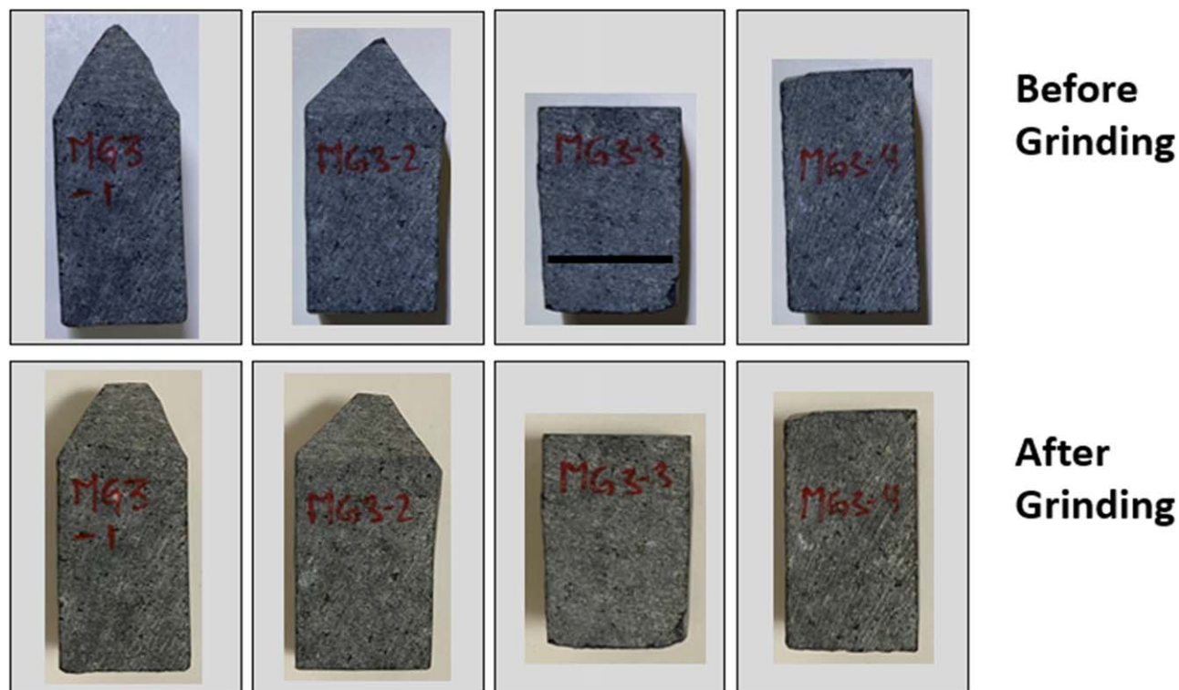
Figure A3. Sample series MG3 clasts before and after grinding. Clasts on the top row are before grinding, and clasts on the bottom row are after grinding. Clasts are approximately 1 cm wide and between 2 and 3 cm tall.
