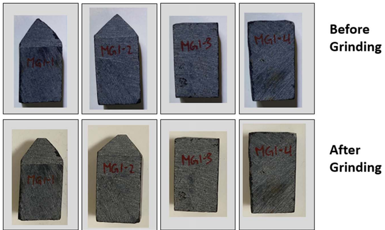
Figure A1. Sample series MG1 clasts before and after grinding. Clasts on the top row are before grinding, and clasts on the bottom row are after grinding. Clasts are approximately 1 cm wide and between 2 and 3 cm tall.
