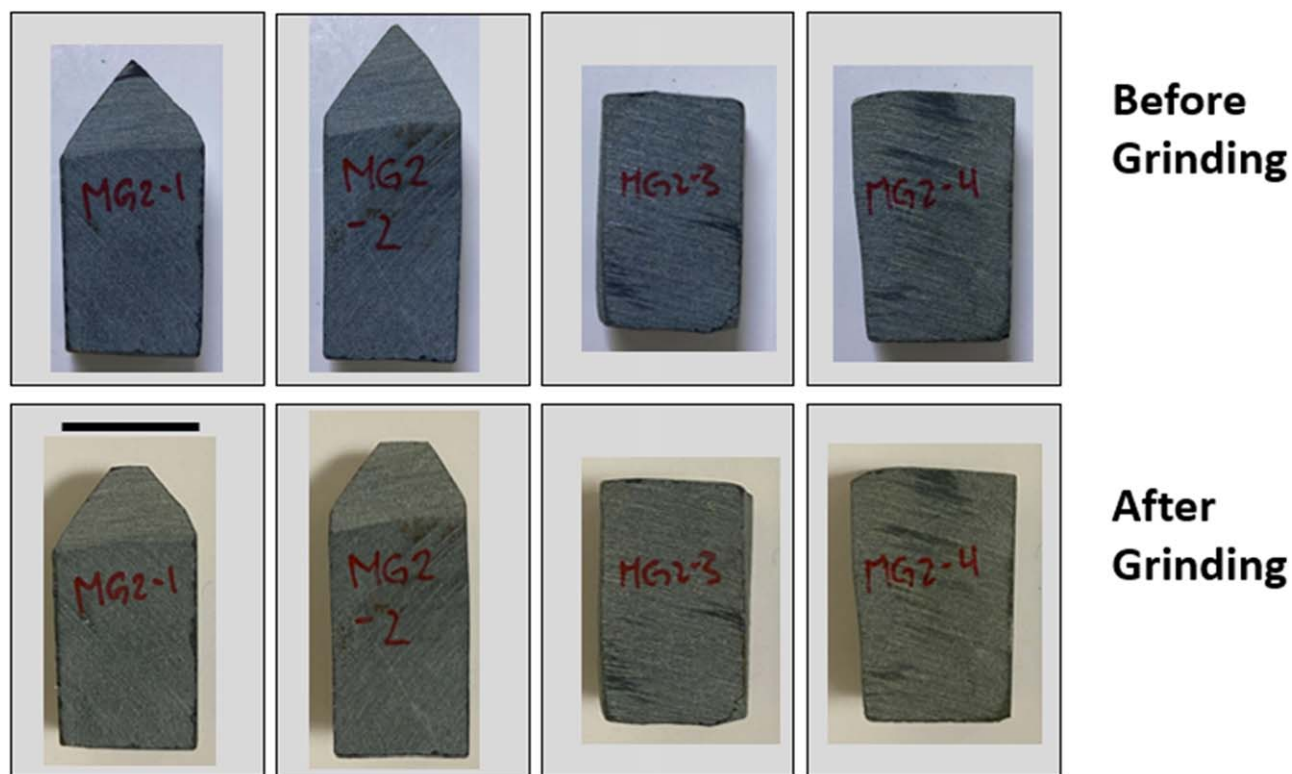
Figure A2. Sample series MG2 clasts before and after grinding. Clasts on the top row are before grinding, and clasts on the bottom row are after grinding. Clasts are approximately 1 cm wide and between 2 and 3 cm tall.
