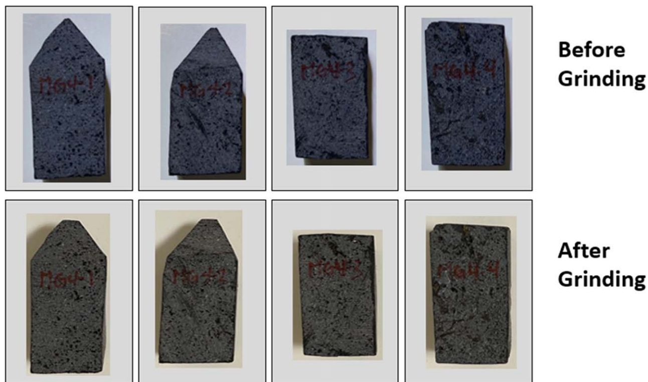
Figure A4. Sample series MG4 clasts before and after grinding. Clasts on the top row are before grinding, and clasts on the bottom row are after grinding. Clasts are approximately 1 cm wide and between 2 and 3 cm tall.
