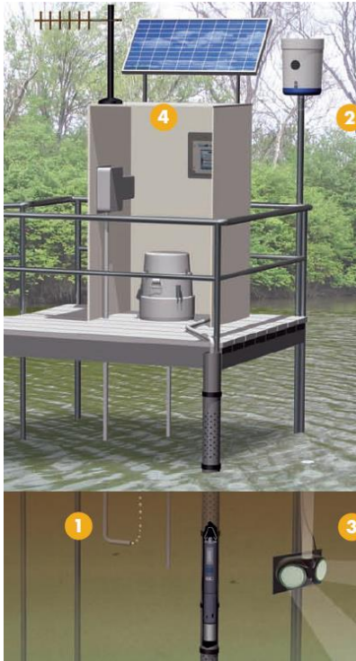
Figure 3-4. YSI flood monitoring and alerting system.
