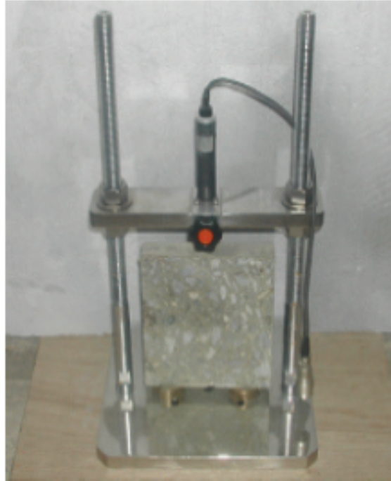
Figure 12: AASHTO-type device of the CTE test, according to Yang et al (2003).
