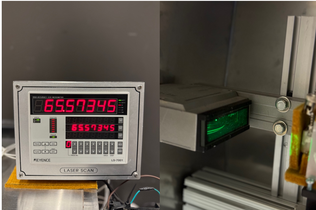
Figure 23: Micrometer and laser beam used for length measurements
