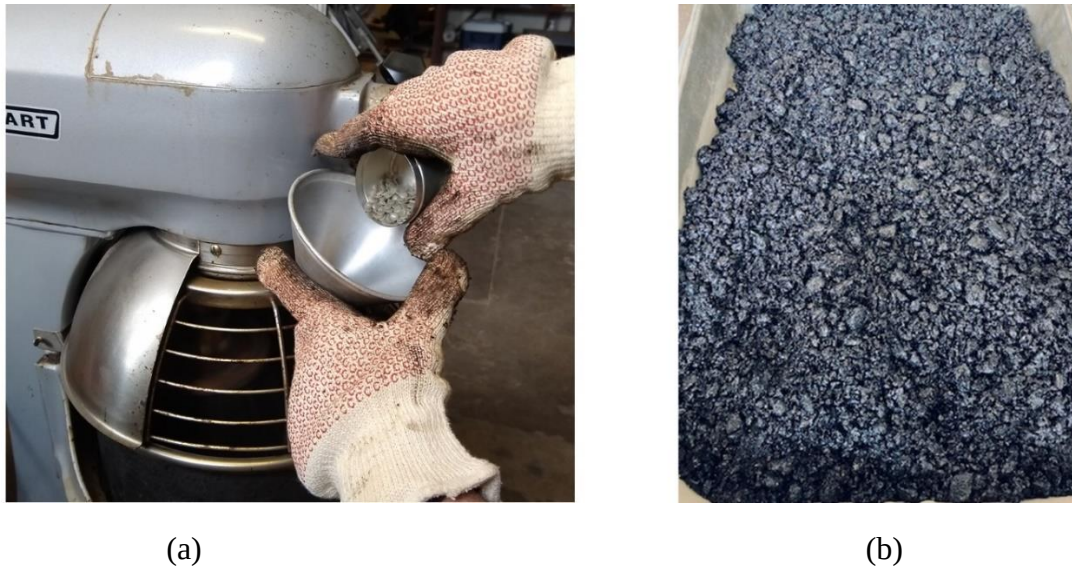
Figure 2.5 Addition of plastic with the heated aggregate-binder mix: (a) Plastic mixing; and (b) Final mix
