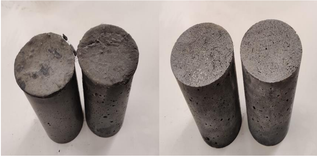
Figure 5. J3 cylinders before and after grinding
