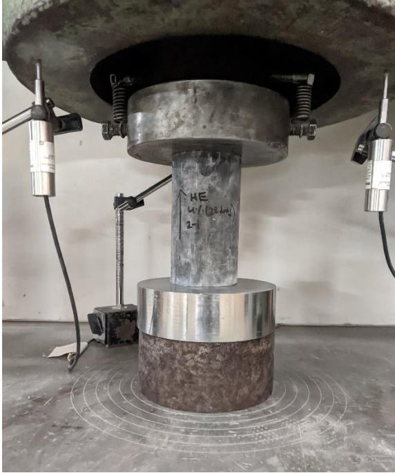
Figure 6. Test setup to measure axial compressive strain.
