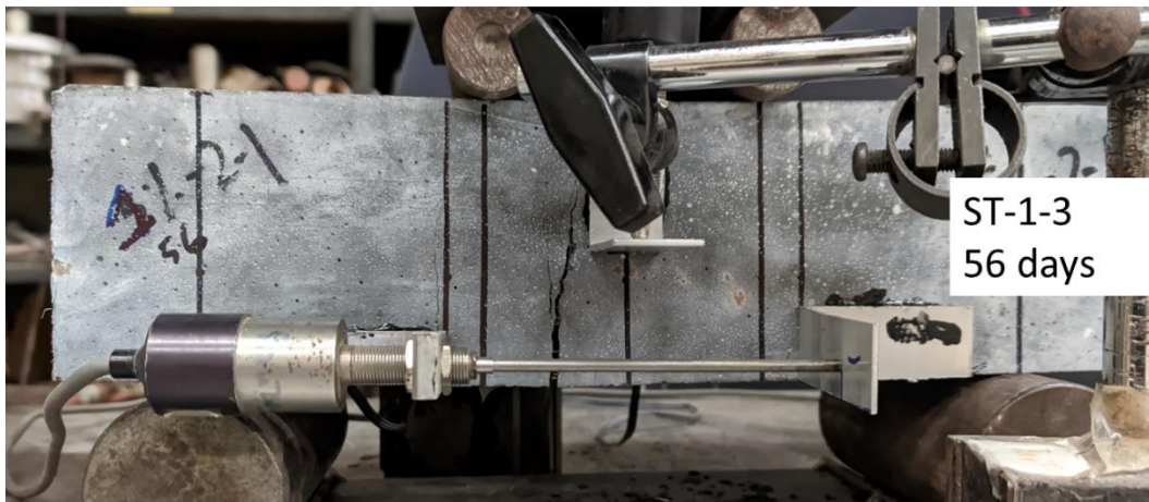
Figure 36. Crack pattern of ST-1% MOR specimens at 56 days age
