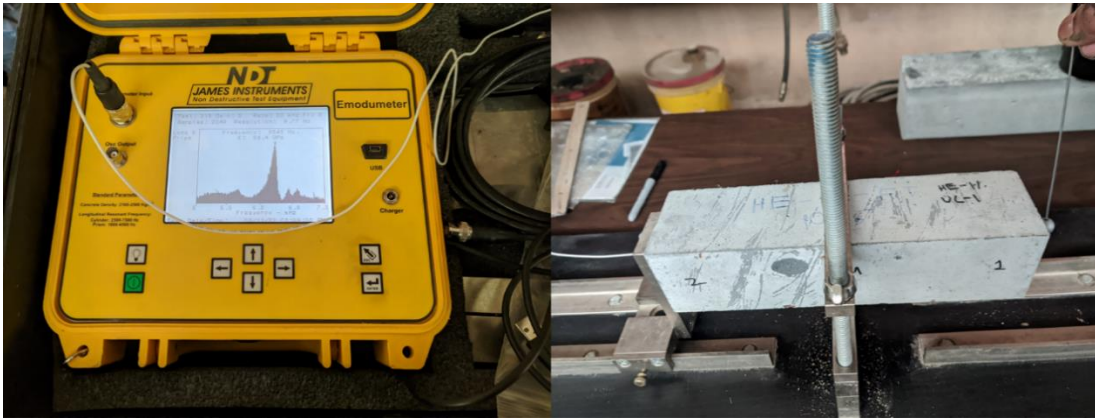
Figure 12. E-Meter device used to generate resonant frequency (left) and test setup to measure resonant frequency of the freeze-thaw specimens (right).
