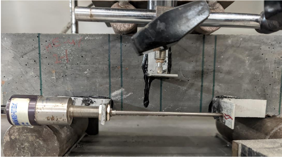
Figure 8. Flexural strength (MOR) test setup
