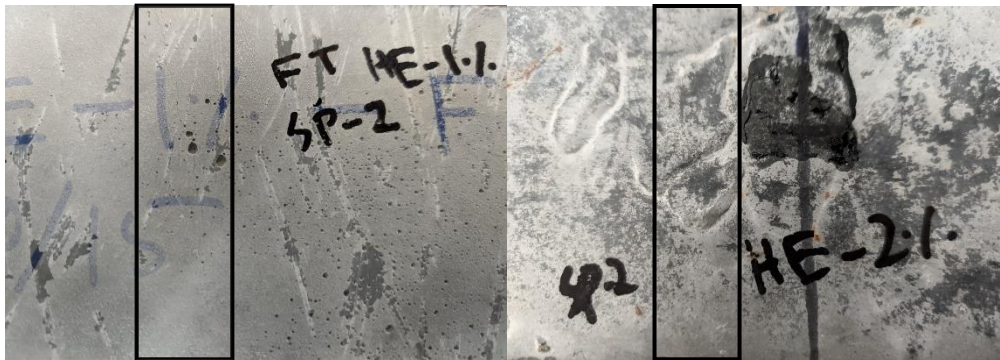
Figure 11. Hairline crack generated in Freeze-Thaw specimens after loading till first load drop for an HE-1% specimen (left) and HE-2% specimen (right)
