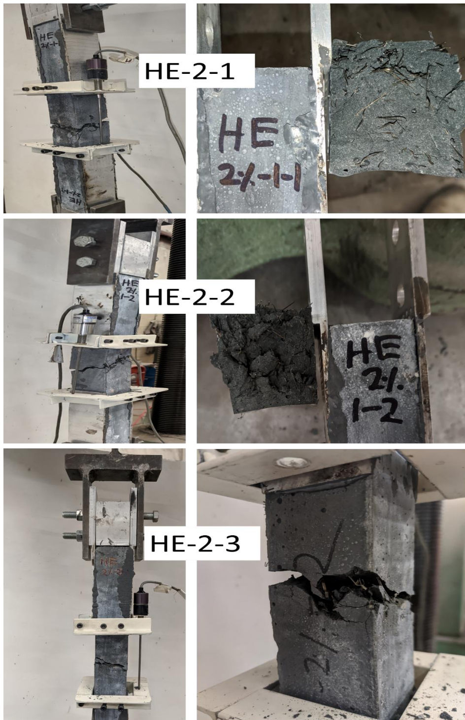
Figure 56. Crack pattern of HE-2% specimens in direct tensile test.
