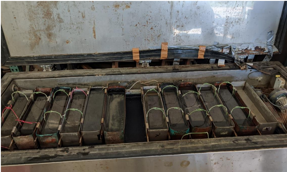
Figure 13. Specimens placed in the freeze-thaw chamber
