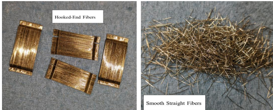
Figure 2. Two types of steel fibers used in this research.
