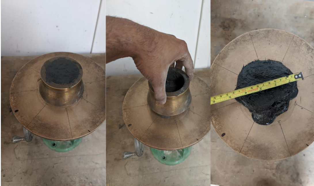
Figure 4. Slump flow test of J3 concrete
