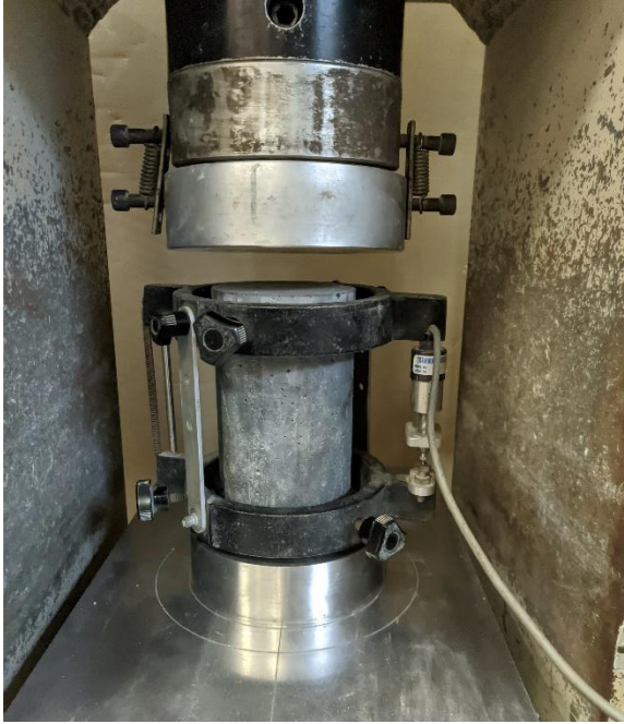
Figure 7. MOE test setup for J3 concrete
