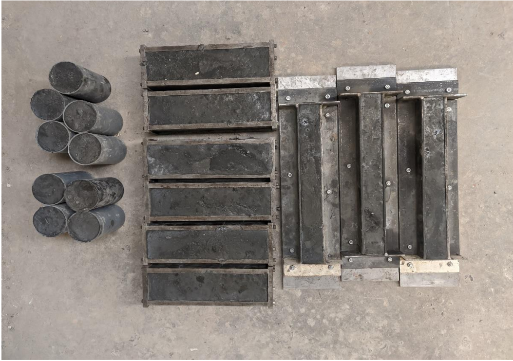
Figure 3. J3 specimens 3 days after casting immediately before demolding.
