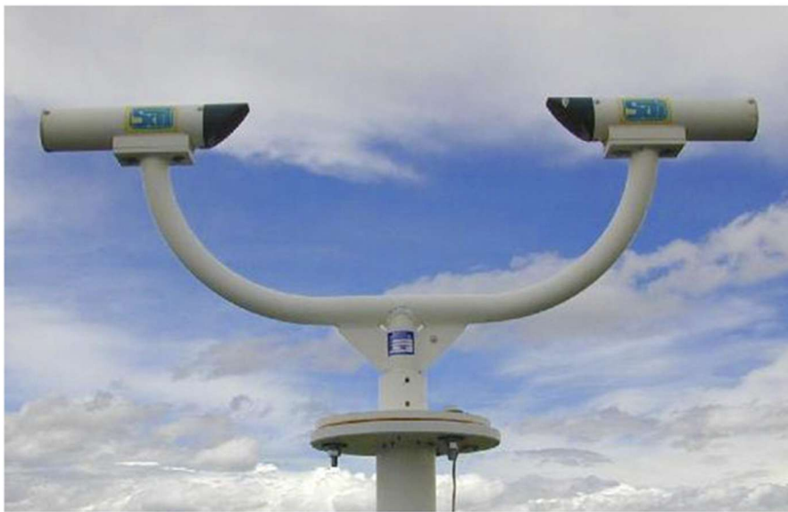
Figure 1: Light Emitting Diode Weather Identifier (LEDWI) that differentiates rain from snow (Photo Credit: Scott Landolt).
