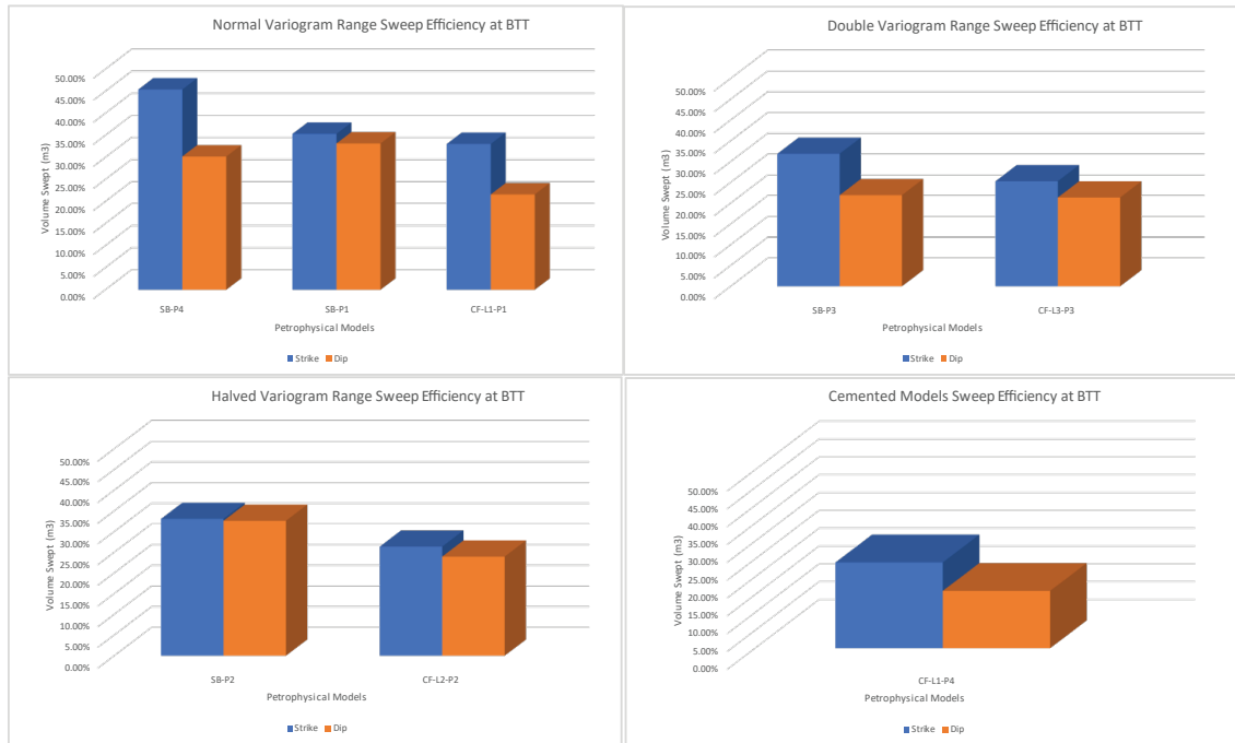
Figure E-2: Charts display comparison of sweep efficiency in each model scenario. Strike direction consistently display higher sweep efficiencies in each scenario at breakthrough time.
