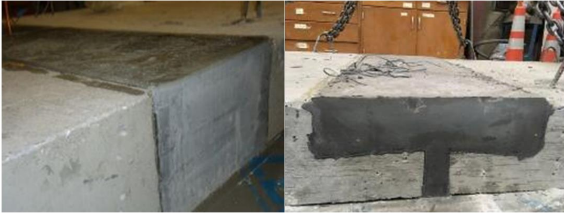
Figure 128. Full-depth (left) and half-depth (right) UHPC connections intended for removal of expansion joints in bridge deck slabs
