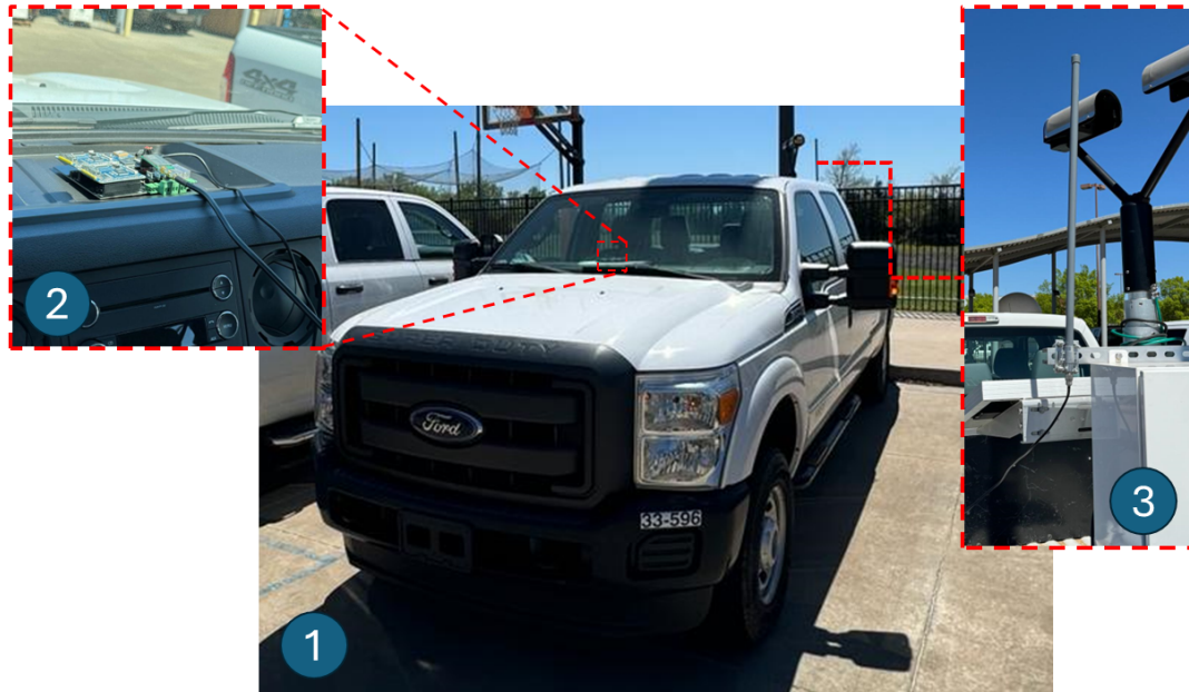
Figure 5.6: Installation of the VSLS PCB in a truck for the range and response time tests: 1. An ARRC truck is prepared for the tests. 2. The VSLS PCB is placed on the dashboard in a way that the internal GPS antenna has a clear line of sight to the sky, and its serial output is connected to a computer to log the data. 3. The same antenna used for the final prototype is mounted on a structure in the bed of the truck.
