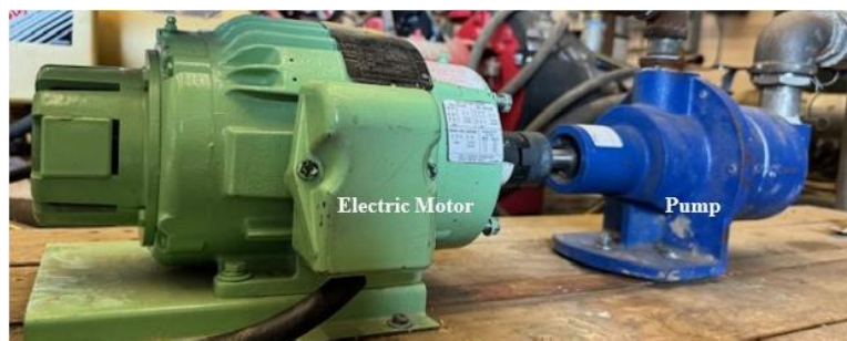
Figure 4.4. Pump Driven by an Electric Motor
