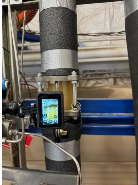
Figure 4.12. Sight Glass, Video Section
