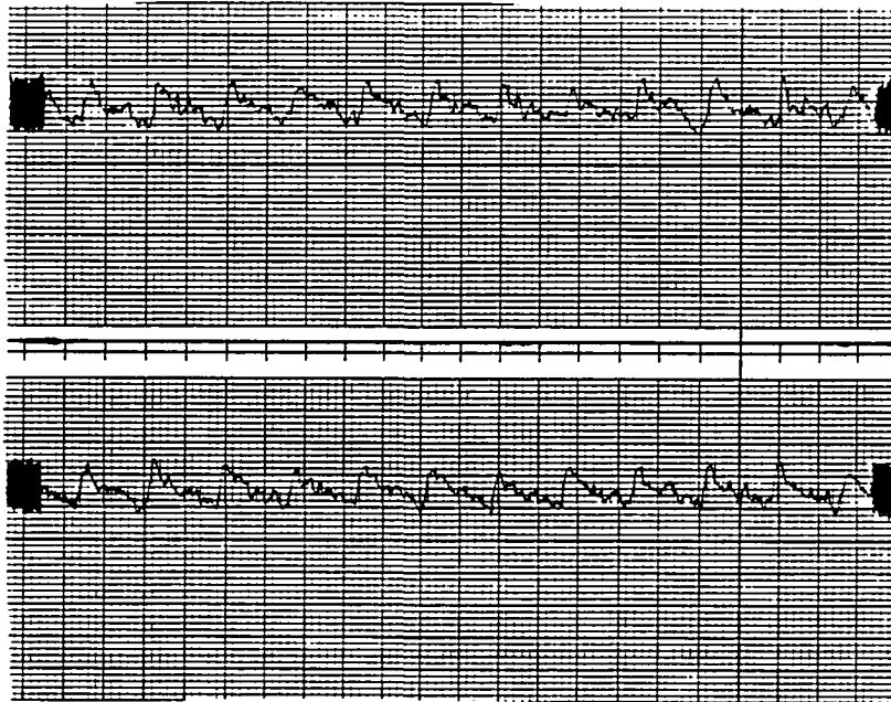
Figure 5.49 An example of Doppler signals recorded from stenotic (25 percent) carotid artery in turbulent flow.
