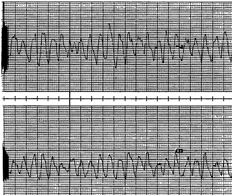
Figure 5.35 The Doppler signals recorded from normal carotid artery for Q_m = 35 ml/min (test J).
