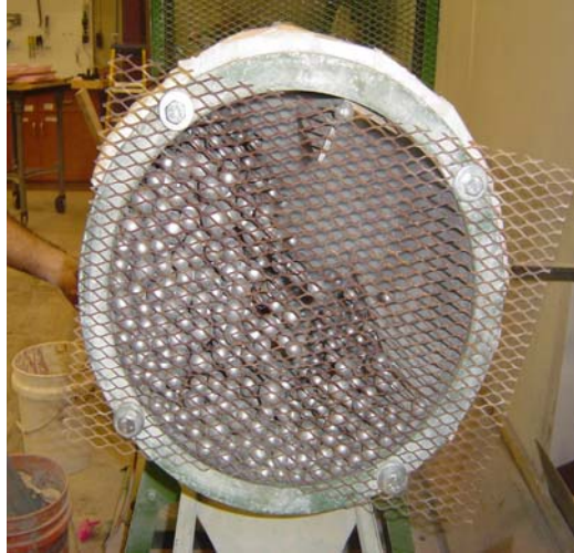
Figure 3.3 Balls motion in the grinding system
