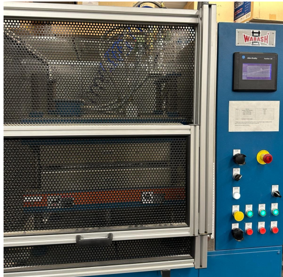
Figure 5.5: Lamination machine with a sandwiched stacked board.
