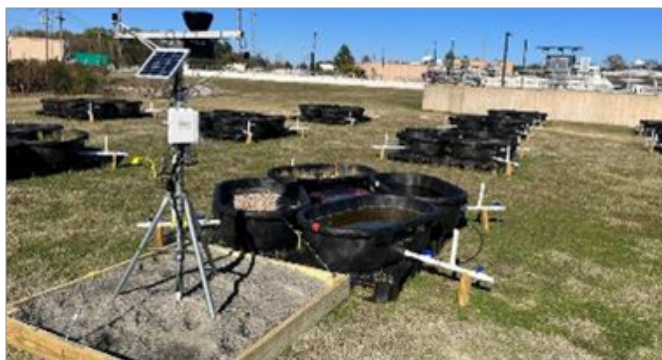
Figure 7.4. HOBO (brand) weather station in operation at the Norman Water Reclamation Facility mesocosm site.
