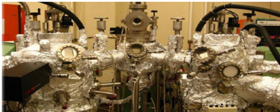
Figure 2-1. Custom two chamber MBE for IV-VI deposition at OU.
