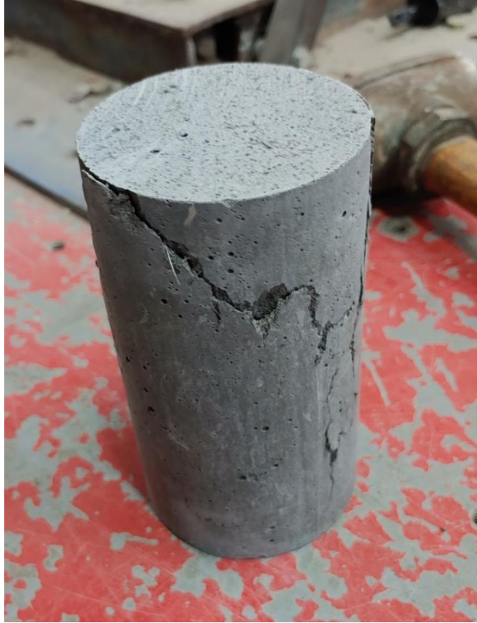
Figure A-5: Broken UHPC cylinder type 2
