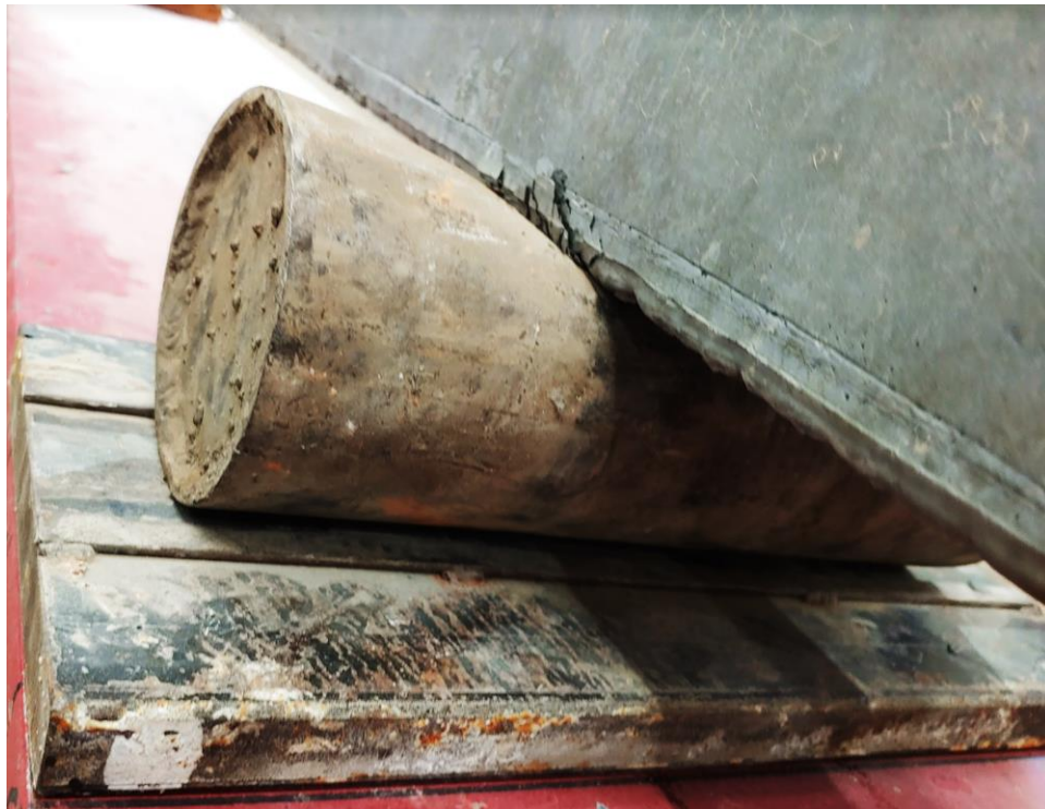
Figure 4-9: Crushed roller under UHPC-B3
