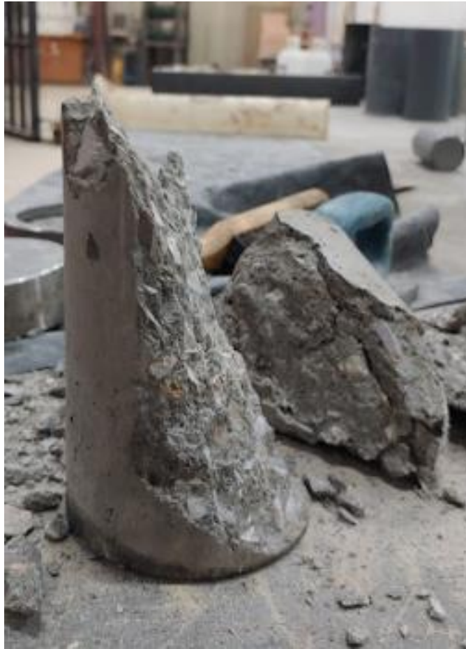
Figure A-1: Broken Class AA cylinder type 4
