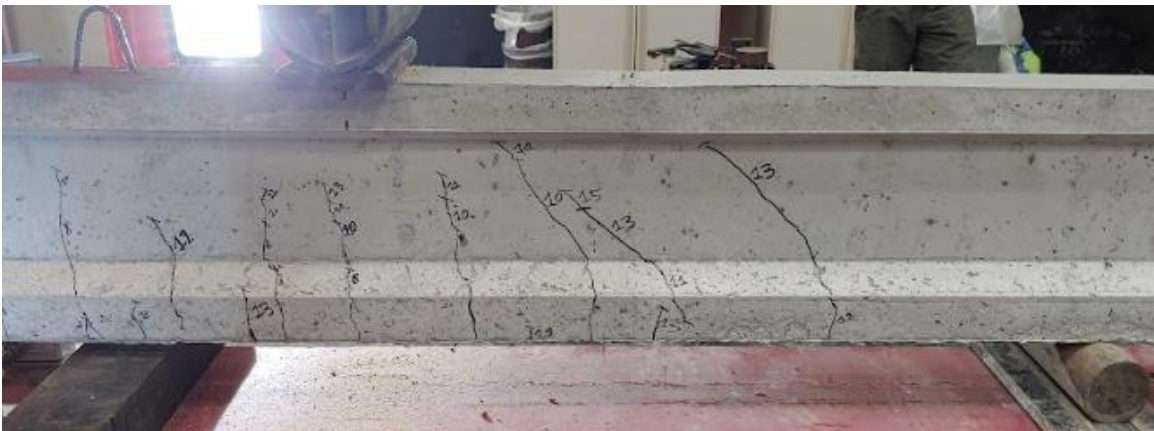
Figure A-26: Flexural cracking in RC-B2 W side
