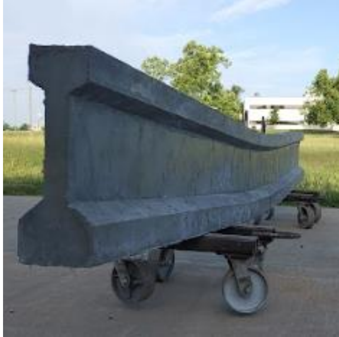
Figure A-51: Permanent deflection of UHPC-B5
