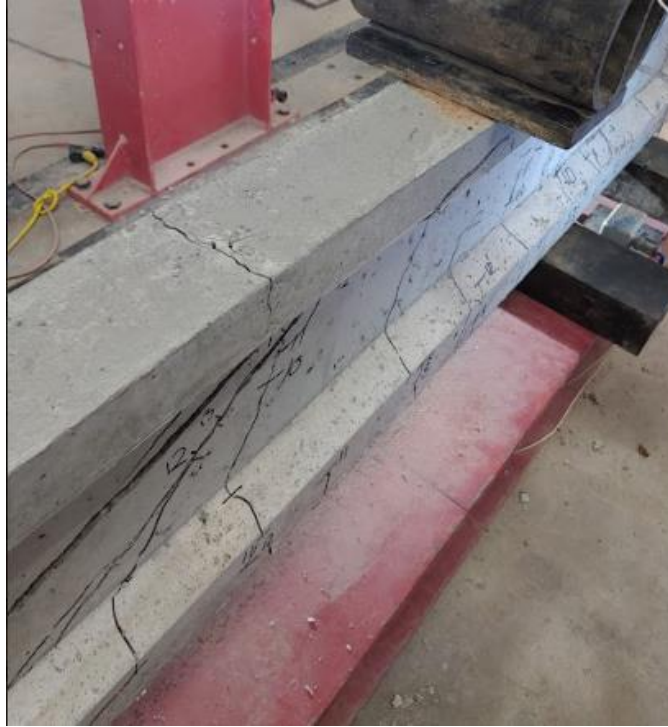
Figure A-27: Buckling of top flange in RC-B2 top view
