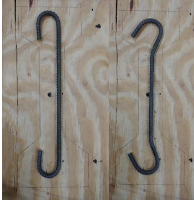
Figure 3-8: Standard stirrup vs. modified
