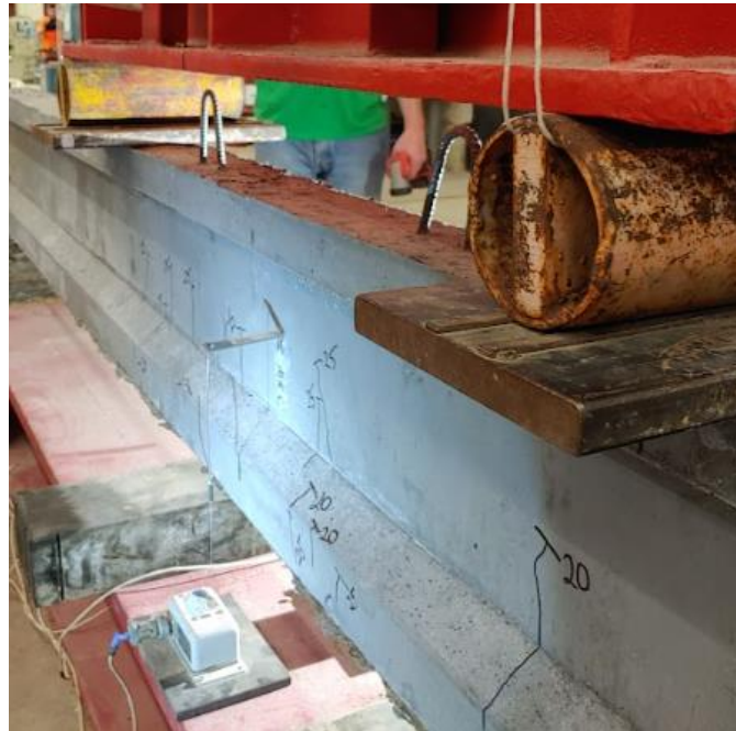
Figure A-38: Top rollers on UHPC-B4 with wider bearing plates
