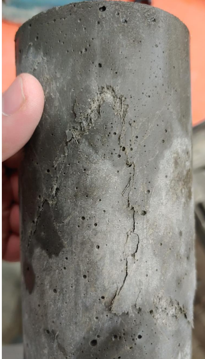
Figure A-6: Broken UHPC cylinder type 3
