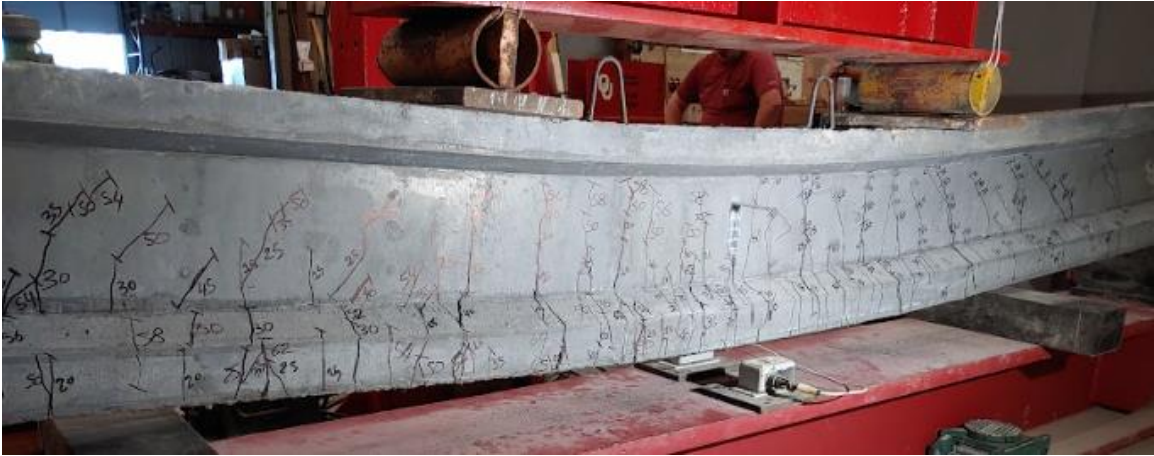
Figure A-47: Cracking in UHPC-B5 SE side
