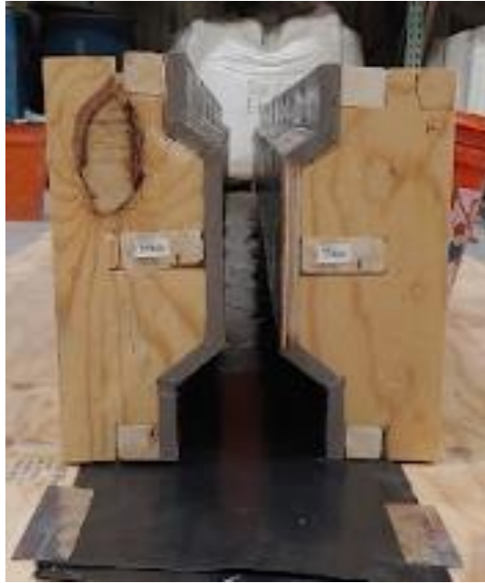
Figure 3-5: Finished sides of formwork
