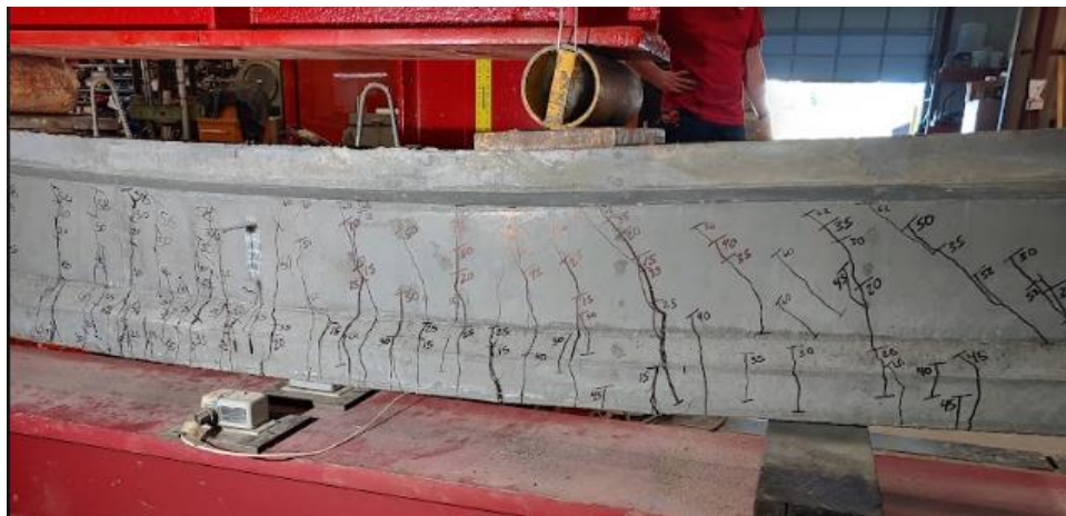
Figure 4-12: UHPC-B3 (a), UHPC-B4 (b), and UHPC-B5 (c) under load
