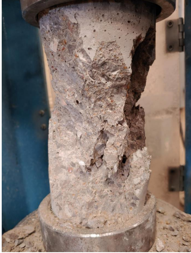
Figure A-2: Broken Class AA cylinder type 1
