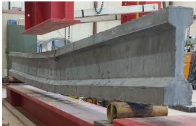
Figure A-34: Deflection of UHPC-B3
