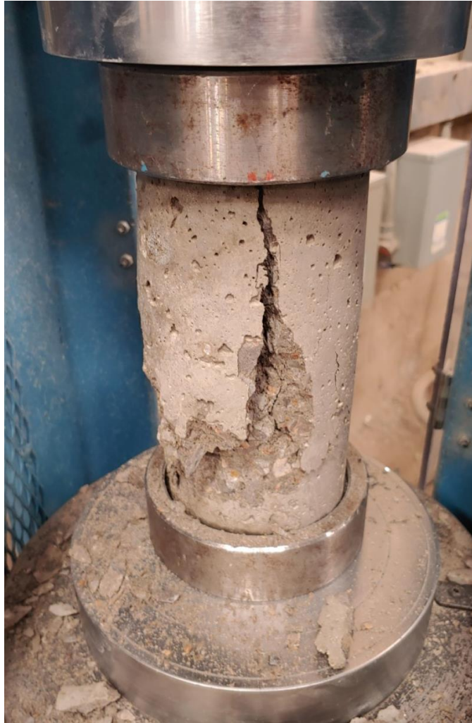
Figure A-3: Broken Class AA cylinder type 2
