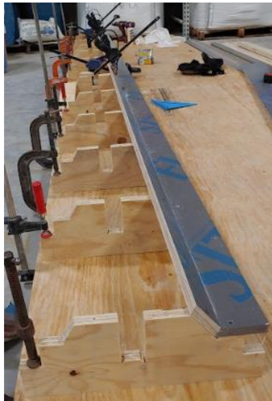
Figure 3-4: Rib pieces in place for face pieces
