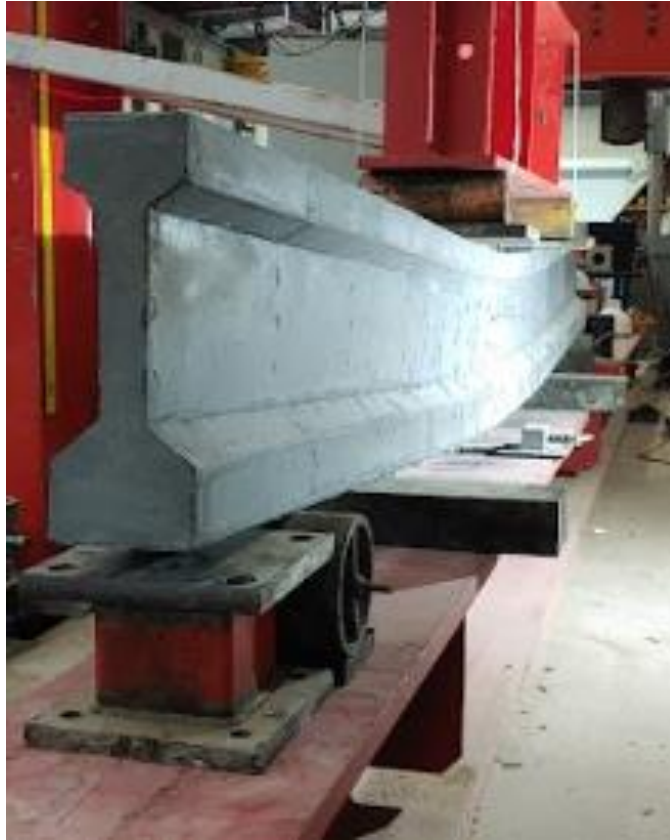
Figure A-45: Deflection of UHPC-B4
