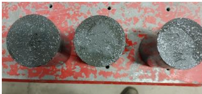
Figure A-4: UHPC cylinders after grinding
