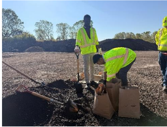
Figure 10: Collection of Asphalt Mix from Plant
