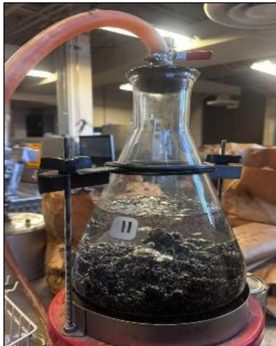
Figure 18: Vacuuming process during the G_{mm} test
