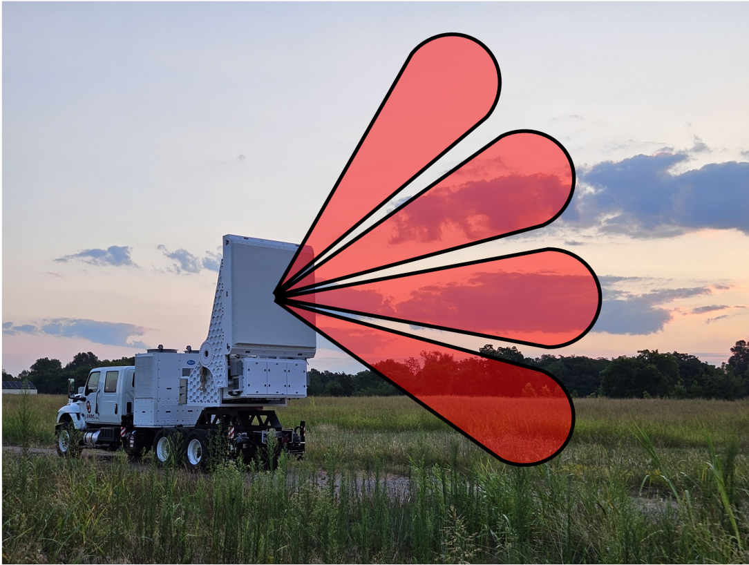
Figure 1.1: Example of Horus forming four spatial beams.
