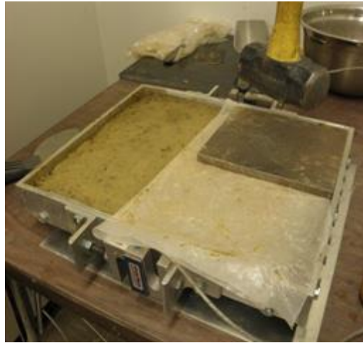
Figure 4.7. Compaction process using a steel plate and a hammer.
