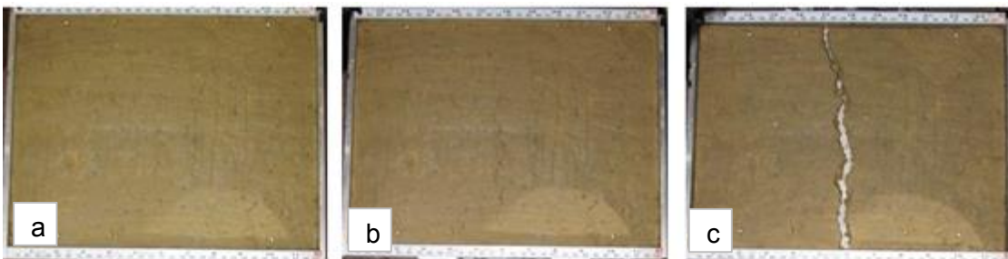
Figure 4.9. Idabel: typical process of desiccation cracking at the beginning of the test (a), 4 hours (b) and 18 hours (c) after starting the test.
