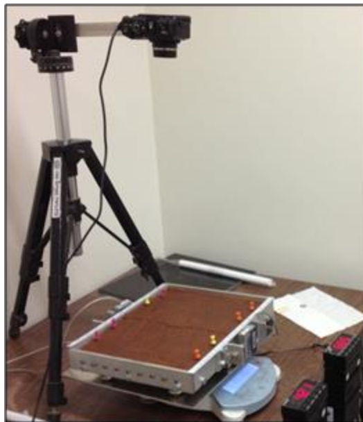
Figure 4.6. Desiccation box test apparatus.
