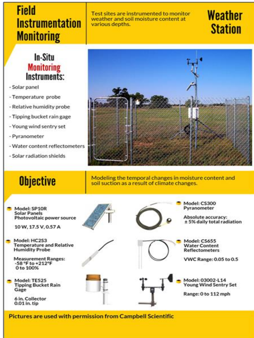
Figure 3.2. Type of sensors and their corresponding range of measurements.
