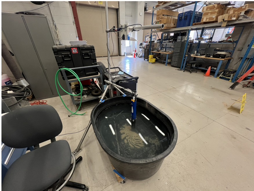
Figure 4.4: Turbidity Experiment Setup
