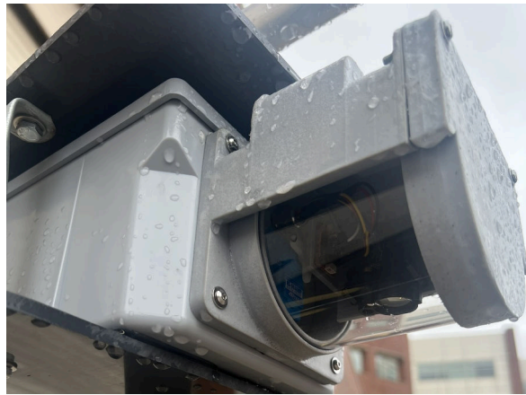
Figure 3.10: Scanning Module After A Rainstorm
