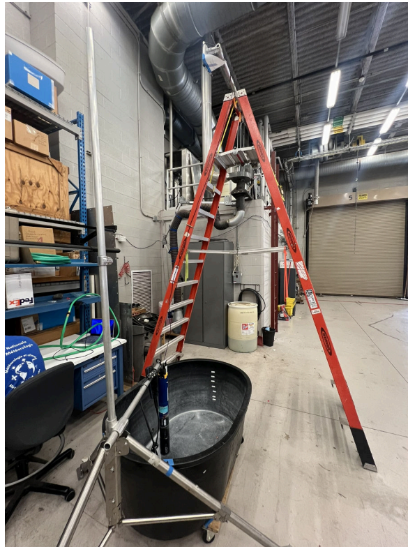
Figure 4.6: Height Increase Turbidity Experiment Setup - Side View
