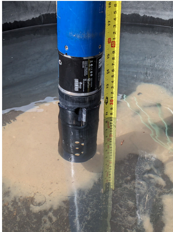
Figure 4.2: Verifying Water Height With Tape Measure
