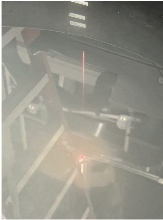
Figure 4.18: Egismos Scanning Through Turbid Water
