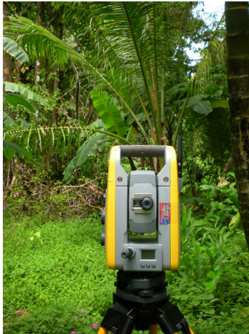
Figure 1.1: Total Station Instrument
