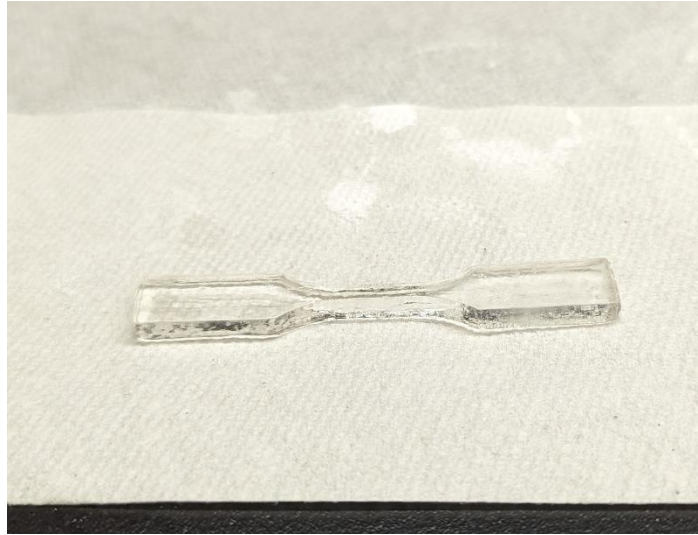
Figure 14: EGDMA Dogbone from rotating platform
