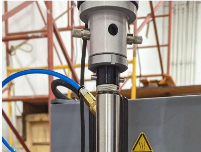
Figure 43: Fabricated adapter connecting the pull rod to the Instron tester
