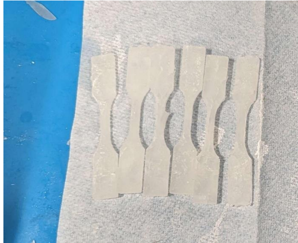
Figure 34: Dogbone synthesis from batch B3G
