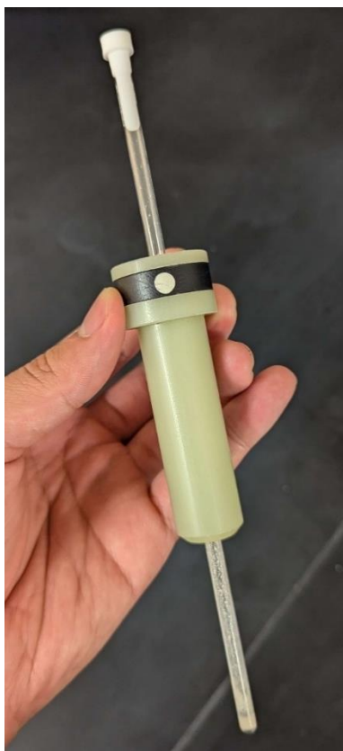
Figure 30: NMR tube containing the sample held by the holder
